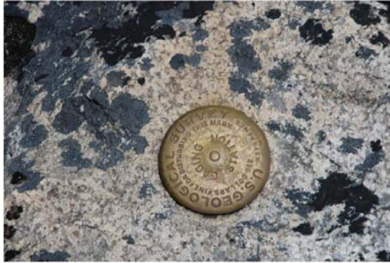
Photo 6. Brass site datum. To be left in place to facilitate future gaging at the site.
