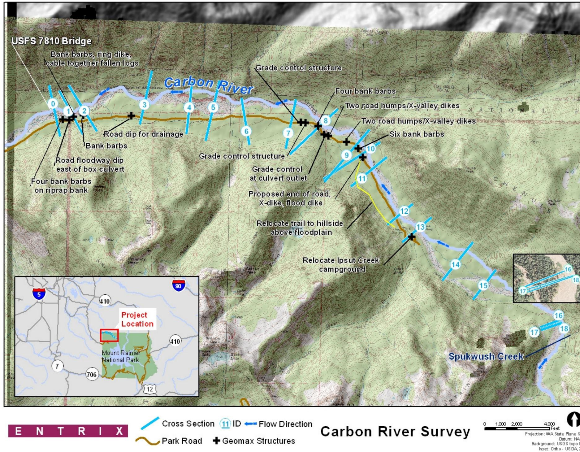
Figure 2. ENTRIX-surveyed cross-sections, September 2008, with location of GEOMAX-proposed flood protection structure
