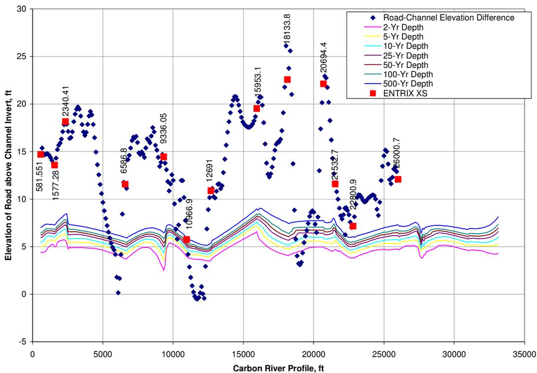
**Figure 18. Elevation difference between the Carbon River road and the river**
