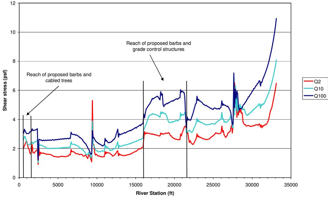
**Figure 9. Carbon River: channel shear stress vs. river station**
