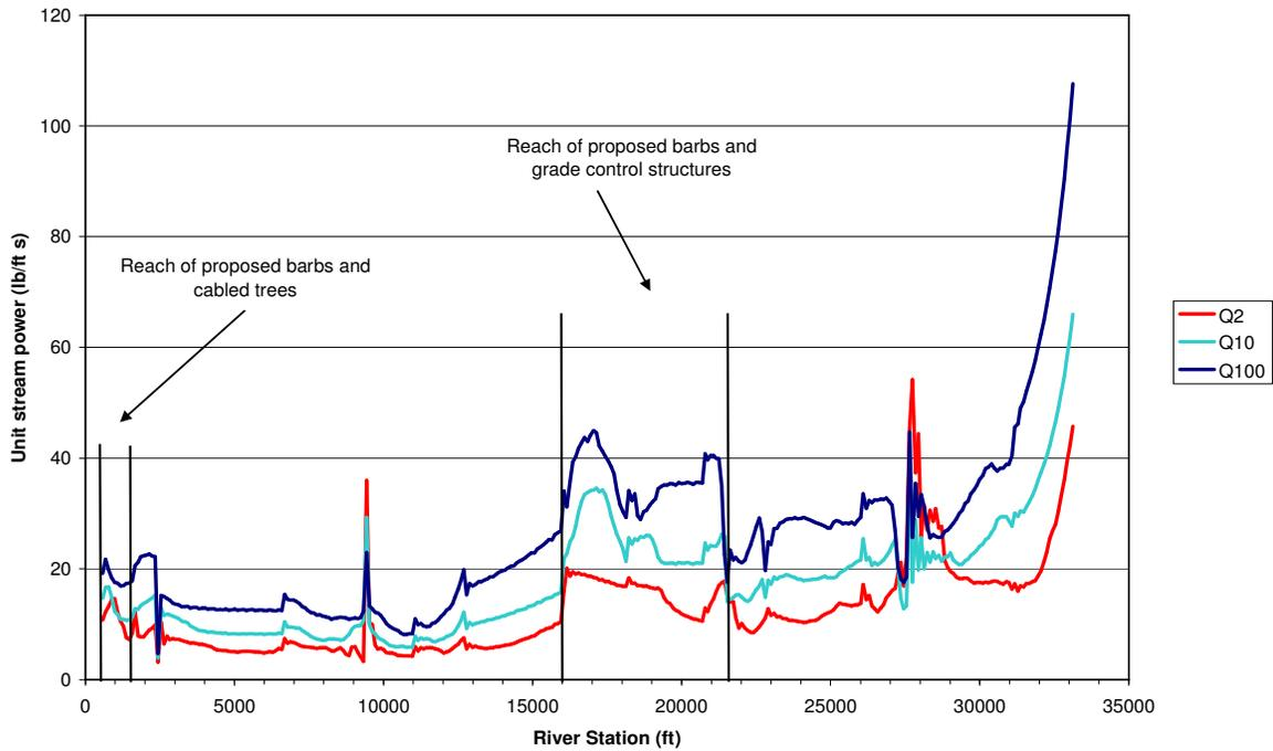
**Figure 10. Carbon River: Unit stream power vs. river station**
