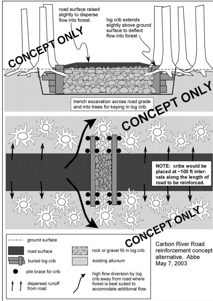
**Figure 16. Rock-filled log crib grade control structure as alternative for protecting road segments subjected to overland flow from river or tributaries**
