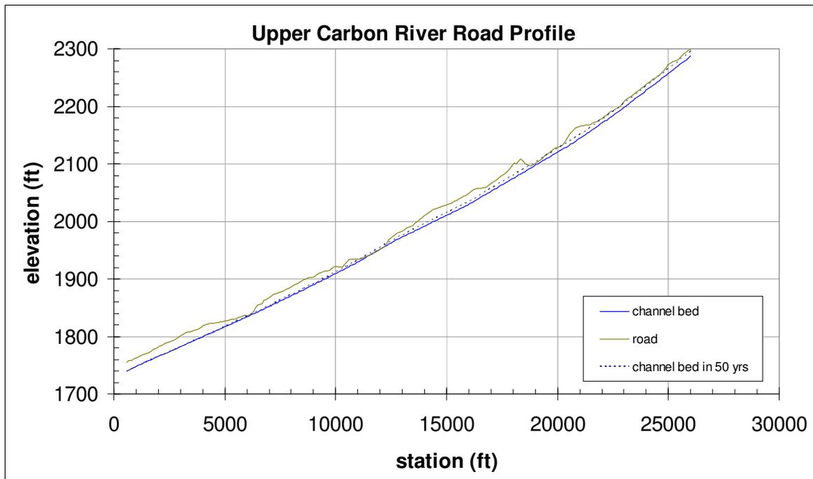
**Figure 21. Upper Carbon River bed profile presently (2008) and estimated in 50 yrs (2058) based on observed trends of aggradation.**
