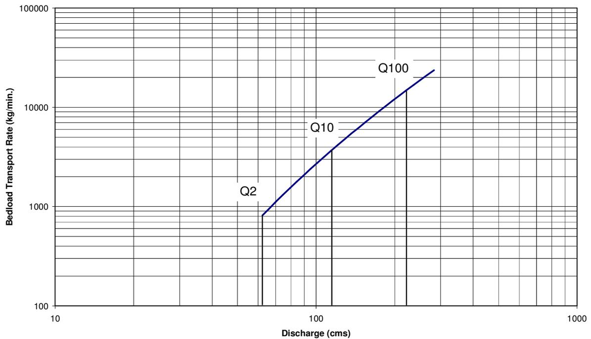
**Figure 12. Carbon River: Uncalibrated estimated sediment rating curve**
