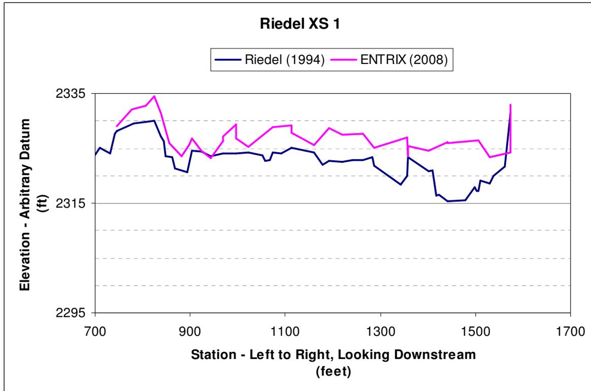
**Figure 11. Representative resurveyed cross-section comparison**
