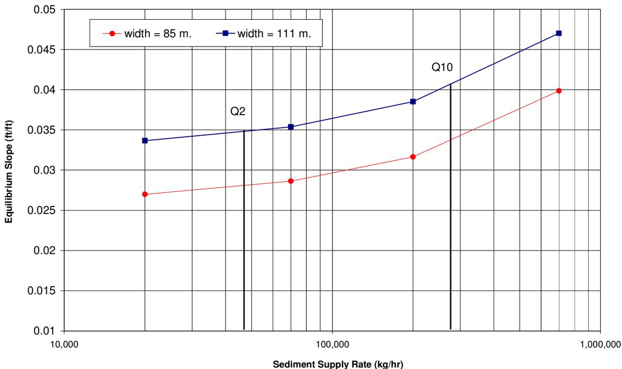
Figure 13. Carbon River: Estimated equilibrium slope as function of sediment supply
