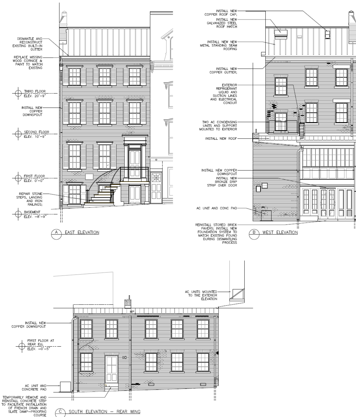
Figure 8. Location of Air Conditioning Condensing Units (Option Considered but Dismissed)
