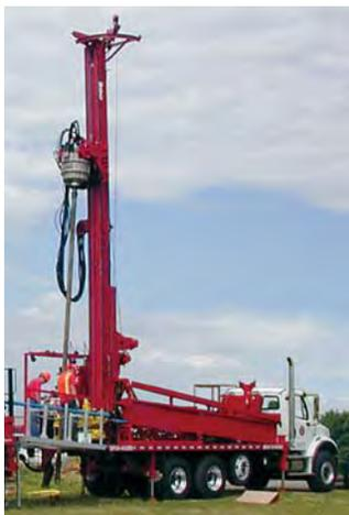
*Sonic drilling rigs, like this one, will soon be in Southeast DC neighborhoods along the prospective tunnel routes to collect soil samples between 150–250 feet deep.*
