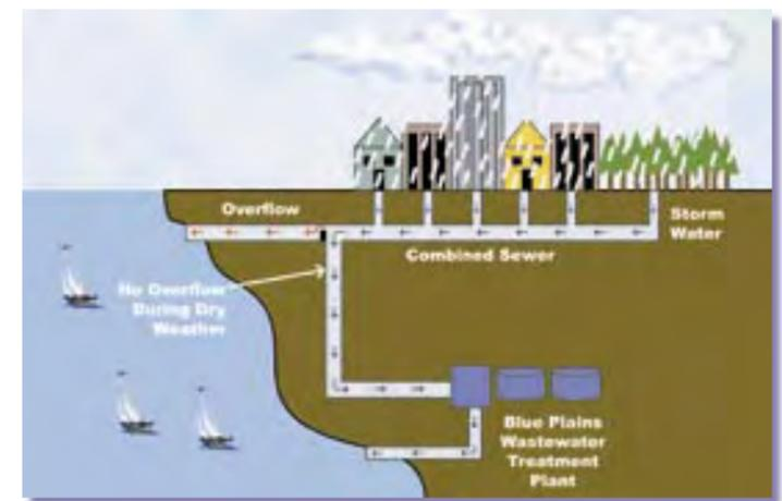
How the District of Columbia's combined sewer system works.
