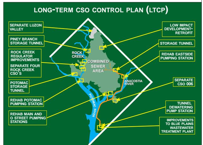
To improve water quality in the Anacostia and Potomac rivers and Rock Creek, the 20-year Long-Term CSO Control Plan includes: three deep underground storage tunnels, including side tunnels to reduce flooding; rehabilitation of existing pumping stations; and the elimination of 14 overflow outfalls. Various sections of this system will be placed in operation along the way to reduce overflows even before the entire project is completed.
