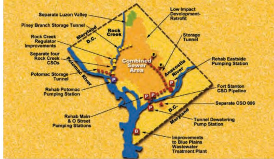
To improve water quality in the Anacostia and Potomac rivers and Rock Creek, the 20-year Long-Term CSO Control Plan includes: three deep underground storage tunnels, including side tunnels to reduce flooding; rehabilitation of existing pumping stations; and the elimination of 14 overflow outfalls. Various sections of this system will be placed in operation along the way to reduce overflows even before the entire project is completed.
