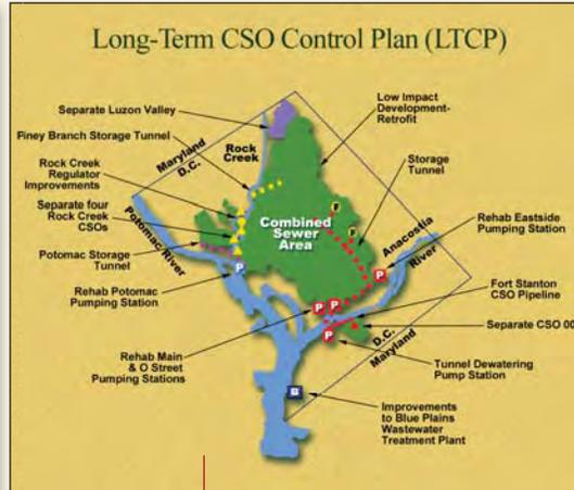
To improve water quality in the Anacostia and Potomac rivers and Rock Creek, the 20-year Long-Term CSO Control Plan includes: three deep underground storage tunnels, including side tunnels to reduce flooding; rehabilitation of existing pumping stations; and the elimination of 14 overflow outfalls. Various sections of this system will be placed in operation along the way to reduce overflows even before the entire project is completed.
