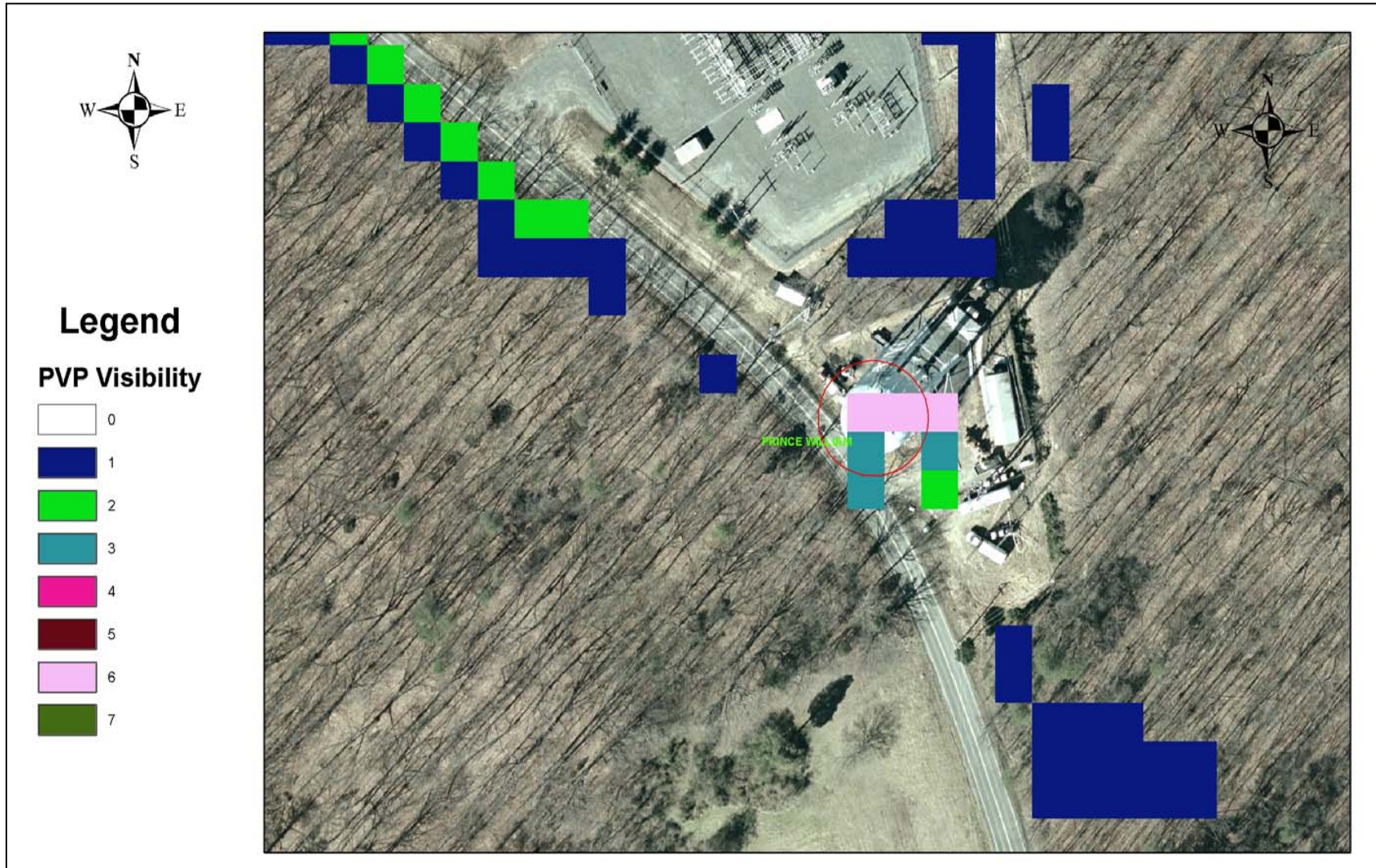
The existing water tower shown above (circled in red) is 148 feet in height and located on Bethlehem Road roughly a half mile south of the battlefield park. The various colors superimposed on the water tower, related improvements and the ground surface reflect the number of PVP viewsheds (from 1 to 6 of 10) from which those site elements would be visible.
