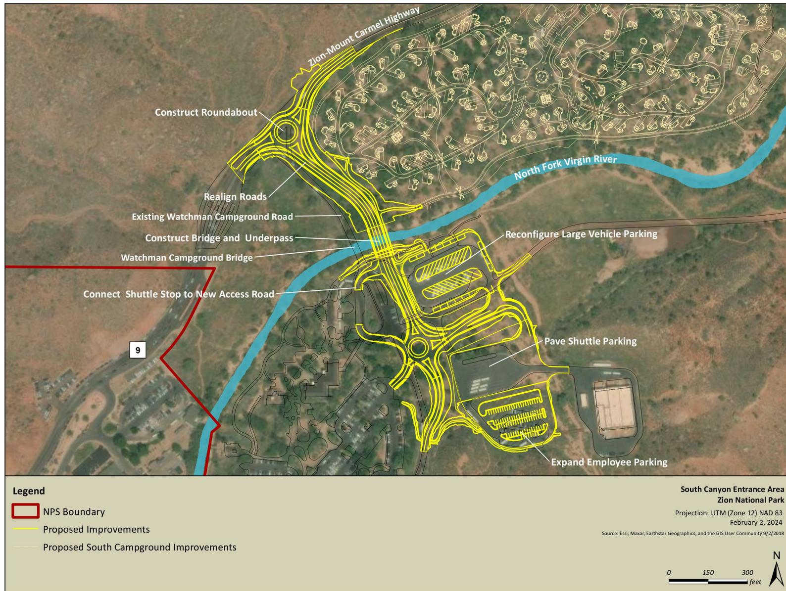
Figure 3. Alternative B – Zion Canyon South Entrance Redesign (NPS Proposed Action and Preferred Alternative)
