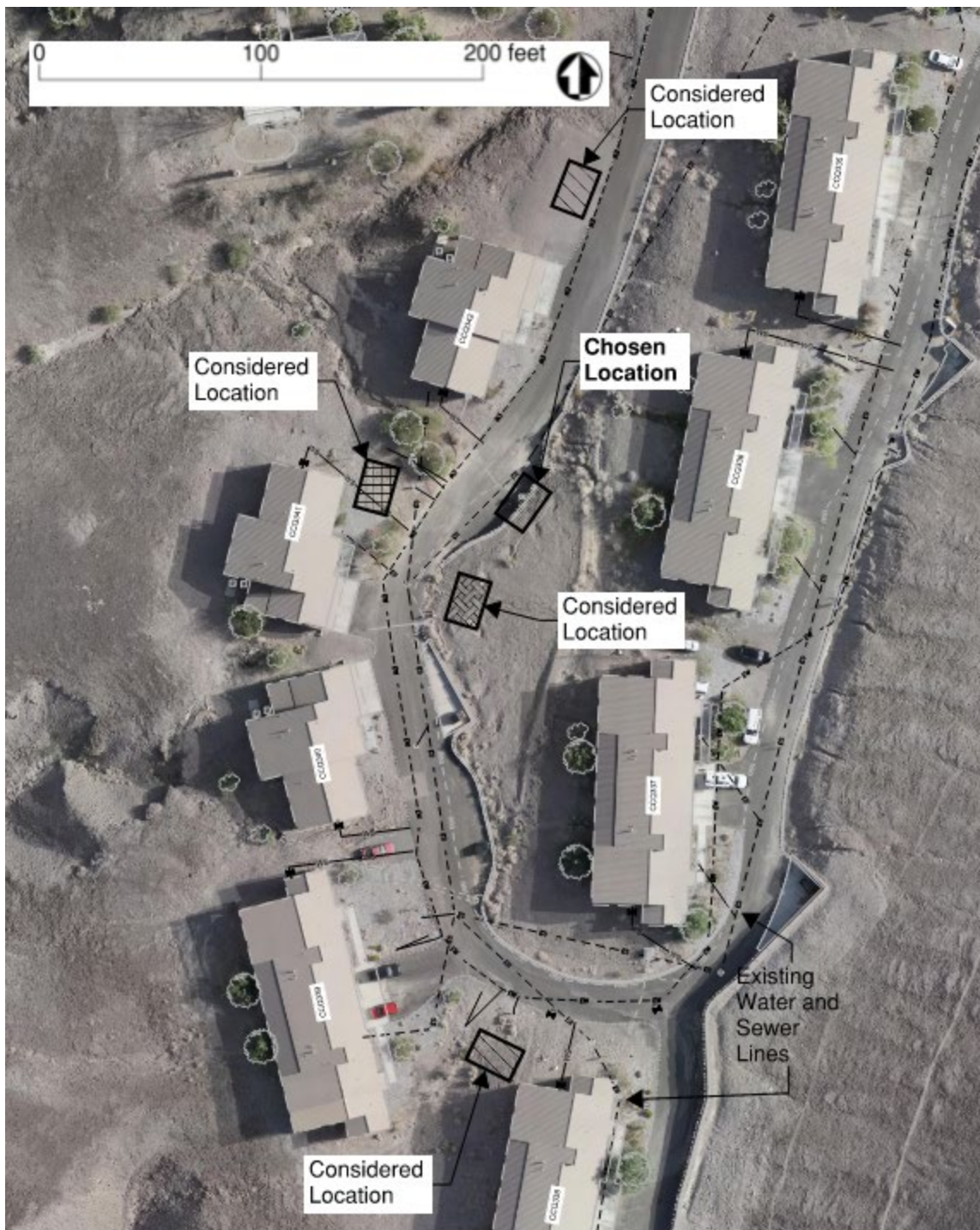
FIGURE A 6 DETAIL ON COYOTE LOOP INCLUDING CONSIDERED AND CHOSEN LOCATION FOR LIFT STATION
