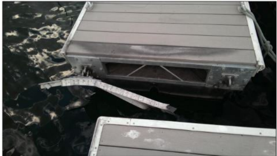
Failed connection to main walkway at end of finger float.
