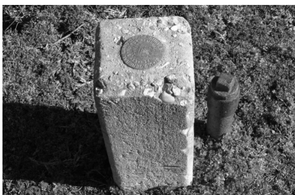
FIGURE 134. A USGS benchmark within the park marking a surveyed elevation. The benchmark is a six inch square concrete post set in the ground, inset on the top with a steel medallion engraved with the survey data.
