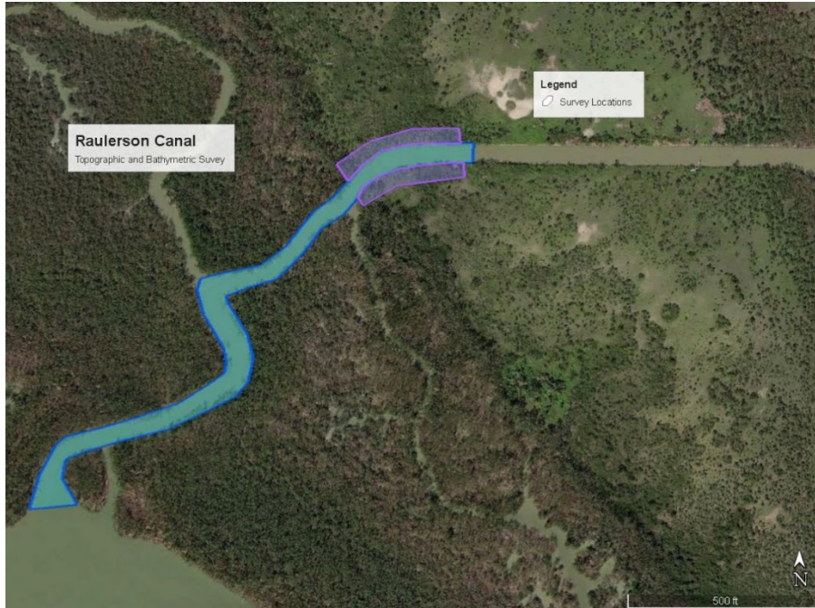
Figure 2. Location of Topographic and Bathymetric Surveys. Topographic surveys will performed in the purple areas. Bathymetric surveys will be performed in the blue shaded areas.
