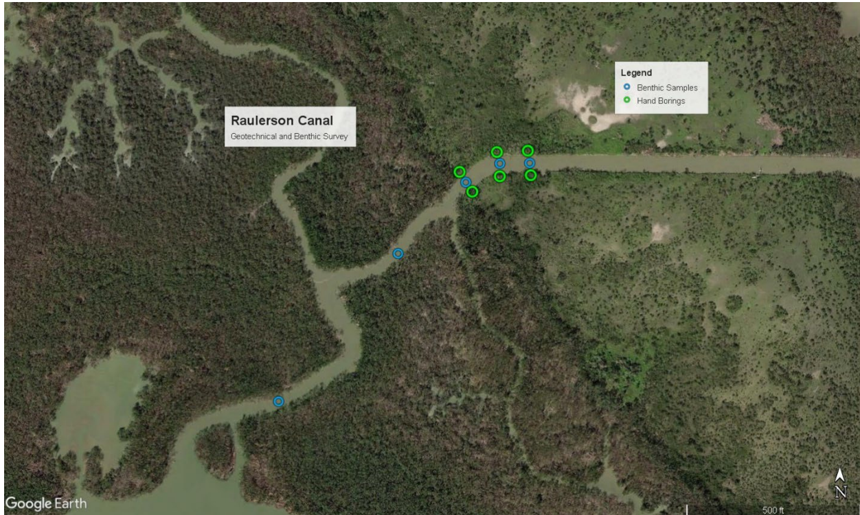
Figure 4. Location of the Geophysical and Benthic Surveys. Geophysical Survey will occur along the 3 transects where the soil borings and benthic samples will be collected in the footprint of the future Raulerson plug.
