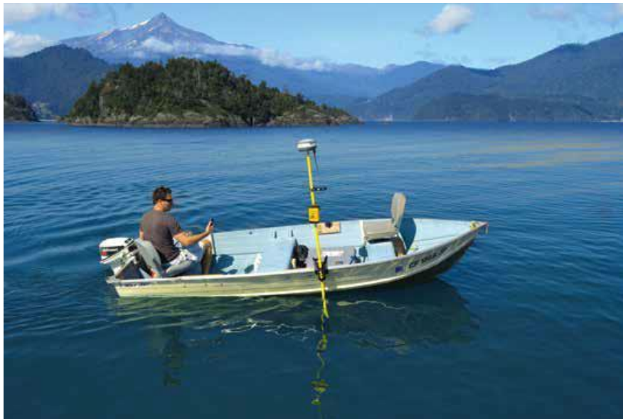
Figure 3. Seafloor Hydrolite DFX dual frequency echosounder mounted on a motorboat
