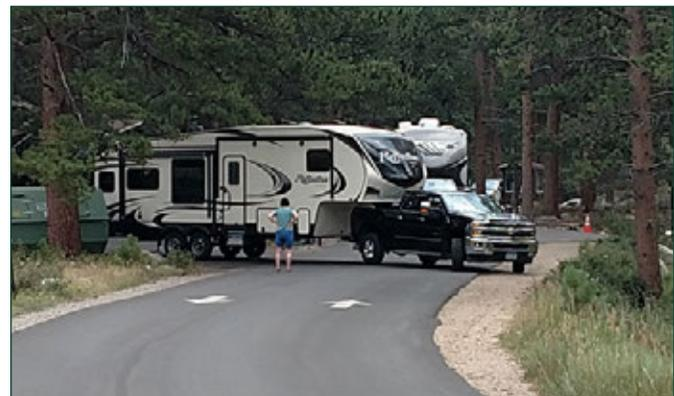
Figure 3.37 Two images show a truck with a fifth-wheel trailer cutting over a radius that’s too small in order to back into a campsite. In this case, a gravel buffer was added to extend the road width without additional asphalt. This assists the driver by providing a widened radius section and protects plant resources on the edge of the road.
