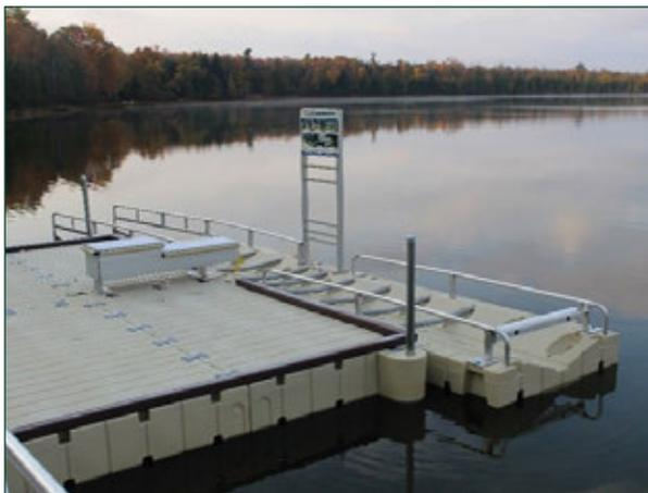
Figure 3.70 Sleeping Bear Dunes National Lakeshore, Michigan, Loon Lake dock. An accessible kayak/canoe launch provides a wheelchair transfer bench, rails to assist getting in and out of the watercraft, and water level adjustment.
