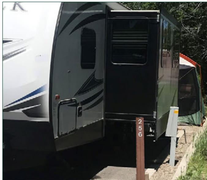
Figure 3.99 Many camper slide outs are located on the same side as the utility hookups. For this reason, additional protection is needed to prevent a camper for inadvertently damaging utilities.
