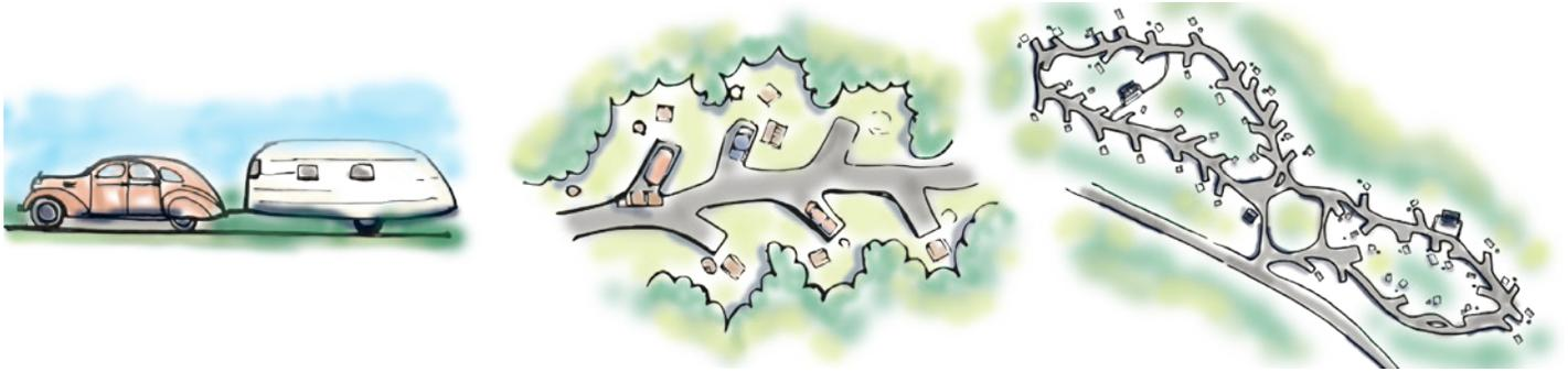
Figure 1.4 1930s to 1940s. The loop campground roads with parking spurs is a signature of 1930s “Meinecke System.” The system included one-way loop campgrounds with parking spurs; rustic style picnic tables and fire grates at every campsite; group amenities provided, including comfort stations, picnic areas, fire rings and water spigots.
