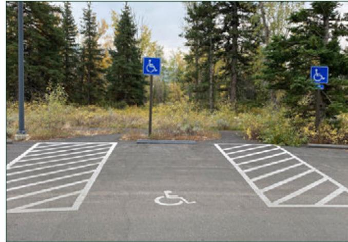
Figure 3.15 Accessible parking space with white parking and white aisle.
