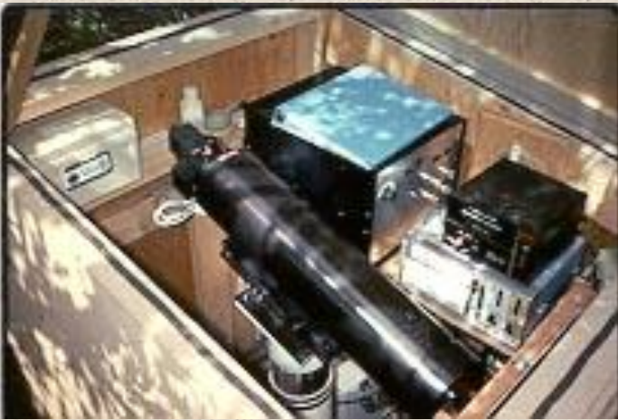
The transmissometer measures visibility conditions from River to Rim at Yavapai Point
