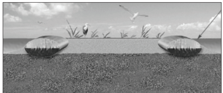
Figure 2. Dam construction using geotubes
