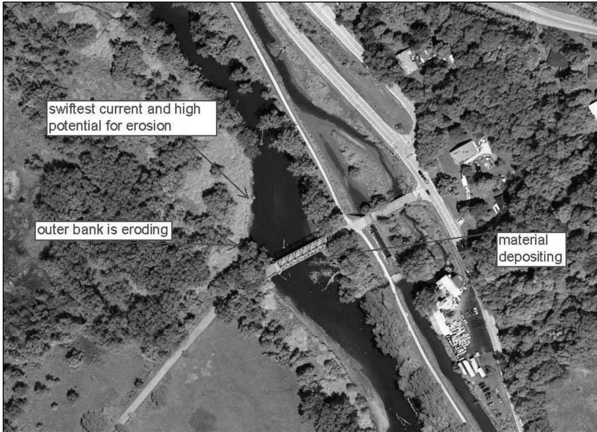
*Figure 13. The erosion patterns surrounding the bridge are shown in this aerial view.*
