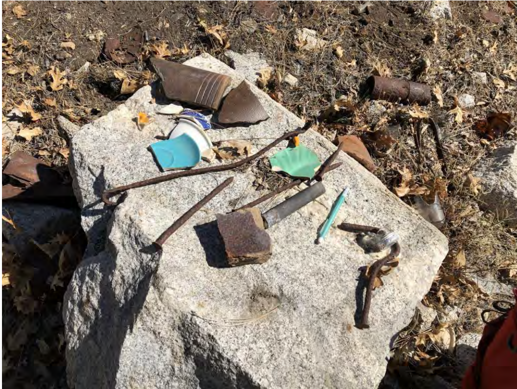
Photograph 9: View of waste fragment types present in soil at the Site, including ceramic, metal, and clay/brick fragments, and an apparent battery core.
