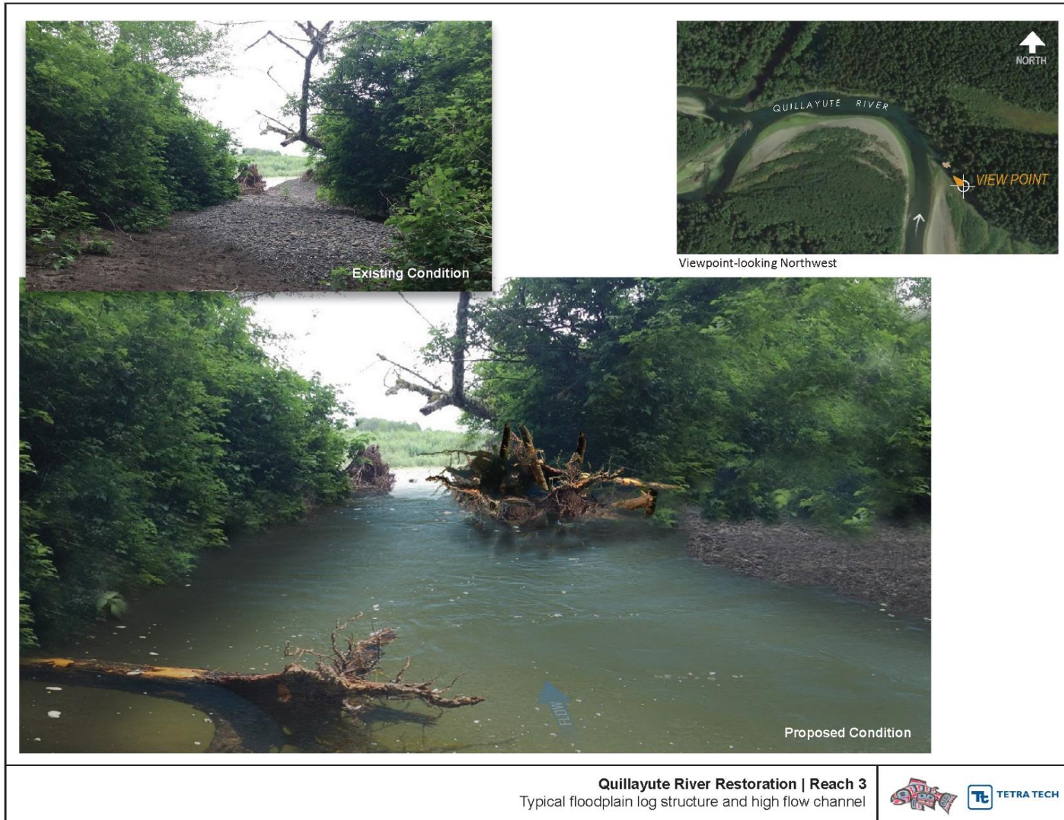
Figure 8. Floodplain Log Structure and High Flow Channel
