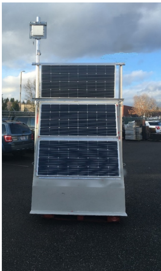
Figure 4. Photo of the actual hut design that would be used on Mount Rainier. Note that the third (top) solar panel would only be used at Ararat South, Copper Mountain, and Mildred Point.
