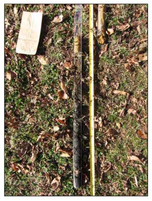
Figure 3. In Boring 1 the surface of the former wetland is marked by dark, viably orgainic deposits below the depth of 11.1 ft. The lowest increment of overlying fill at the depth of 9.7 ft is also darkly colored and contains coal, broken glass, and a fragment of rubber seal, probably that of a mason jar.
