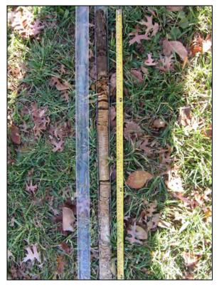
Figure 2. The upland soil of Boring 4 has suffered some agricultural deflation or shallow grading, but is not as disturbed as those of two other examined locations. Grayer colors near the base of the core are due to drainage mottling. Soil drainage is, however, not sufficiently impeded to restrict occupation.
