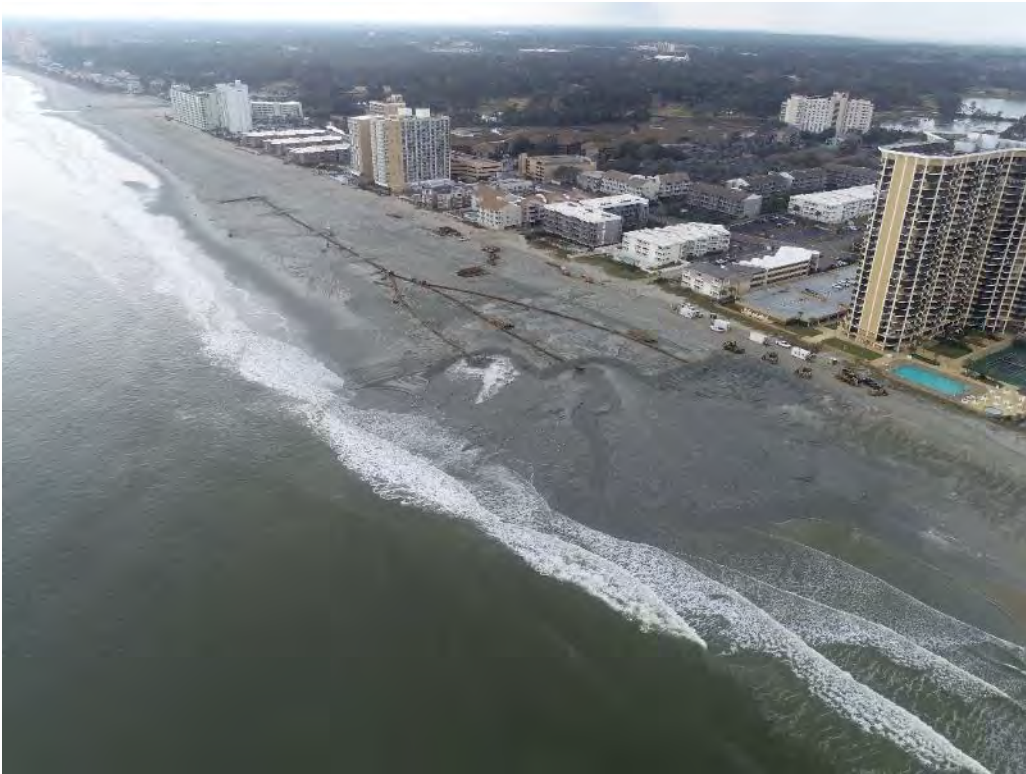
Figure 6. Aerial of onshore beach nourishment setup depicting elbow pipe (Image credit: CSE)
