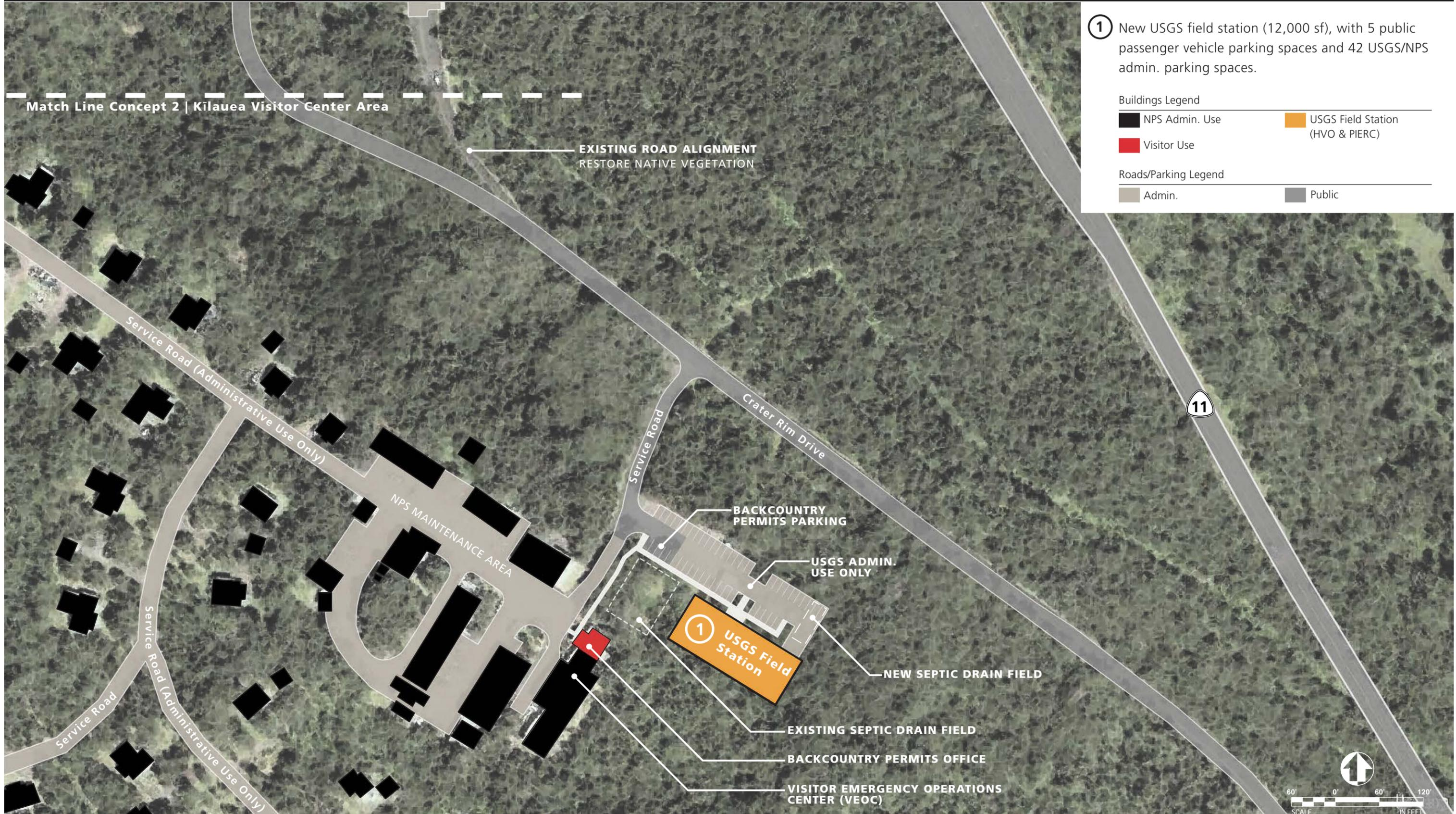
① New USGS field station (12,000 sf), with 5 public passenger vehicle parking spaces and 42 USGS/NPS admin. parking spaces.
