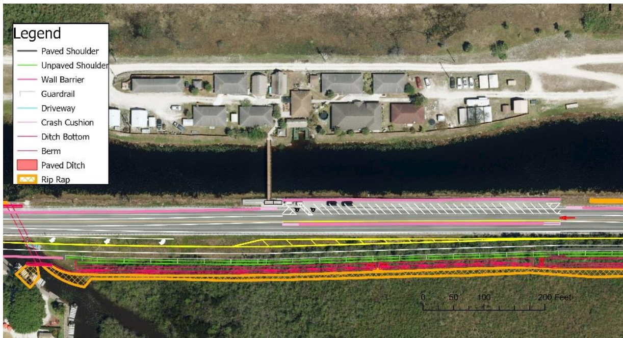
Figure 10. Proposed diagonal parking and new access lane added at the Miccosukee Tigertail Camp.
