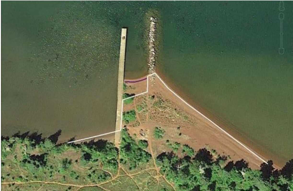
Figure 11. Satellite Imagery of Siskiwit dock (2013) showing accretion between the dock and breakwater but no change to the fillet beach. White line shows 1992 shoreline. Dark purple line shows 2009 shoreline.
