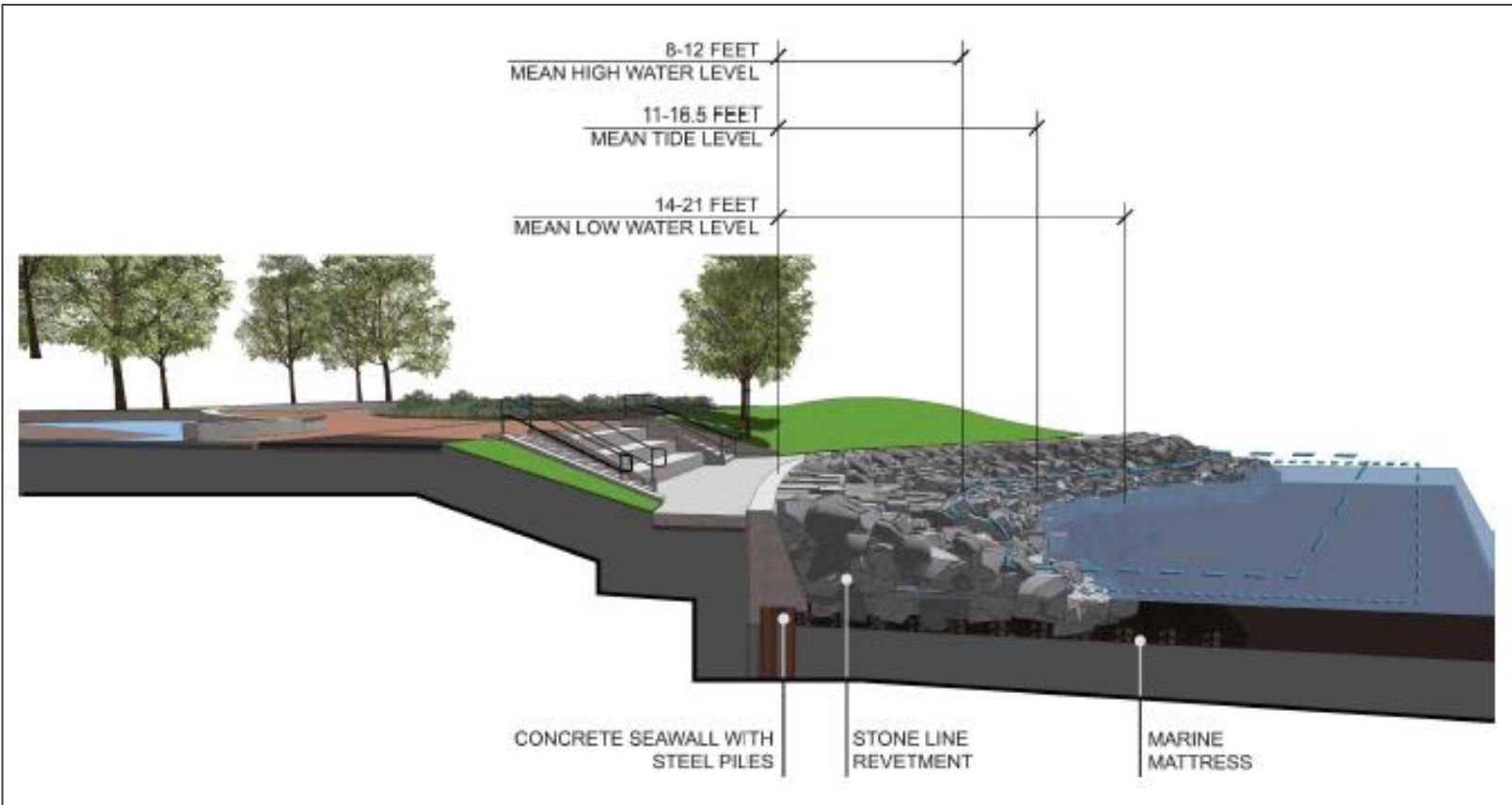
Figure 4: Cross-section of Option 1 showing concrete stair access to a lawn area and the seawall, with revetment to the mean tide mark.
