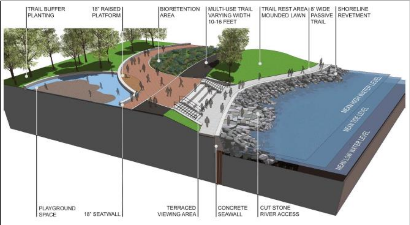
Figure 5: Cross-section of Option 1 showing the proposed play areas, multi-use trail, and stair access to a lawn area, seawall, and revetment.
