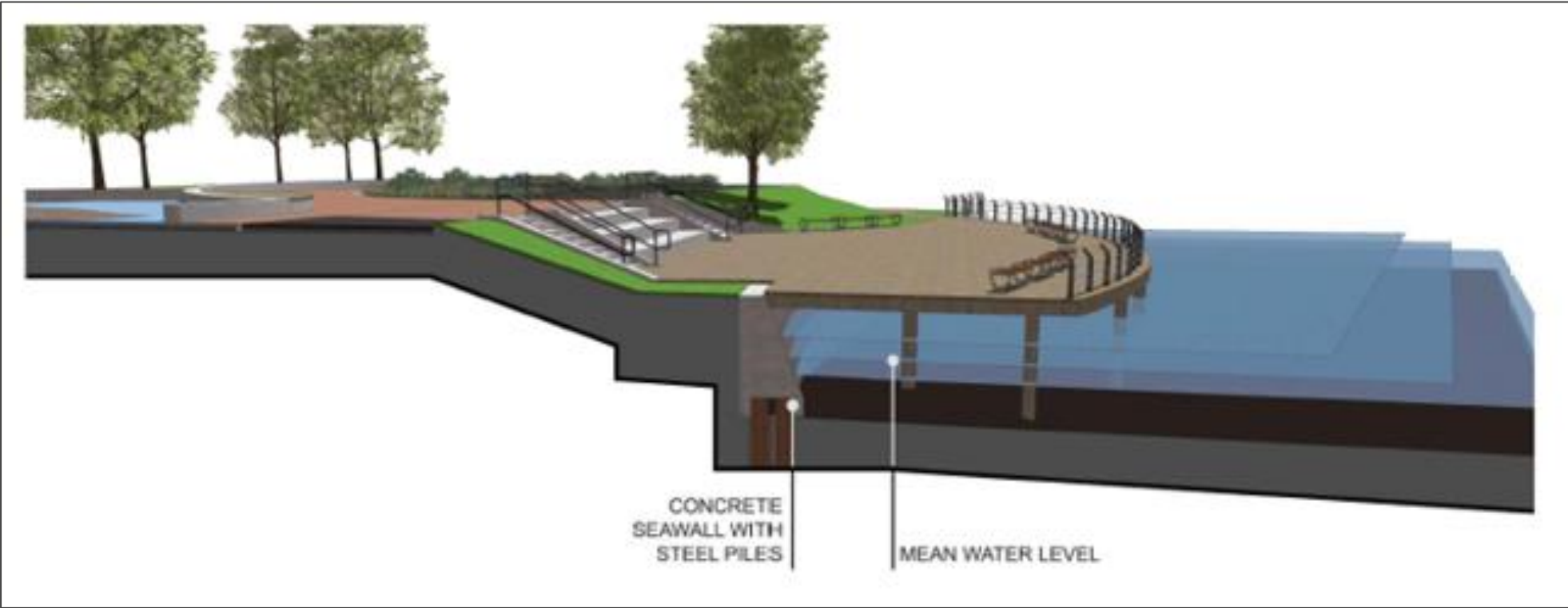
Figure 8: Cross-section of Option 2 design showing a play area, bioretention area, multi-use trail, mounded lawn, and an overlook of the river.
