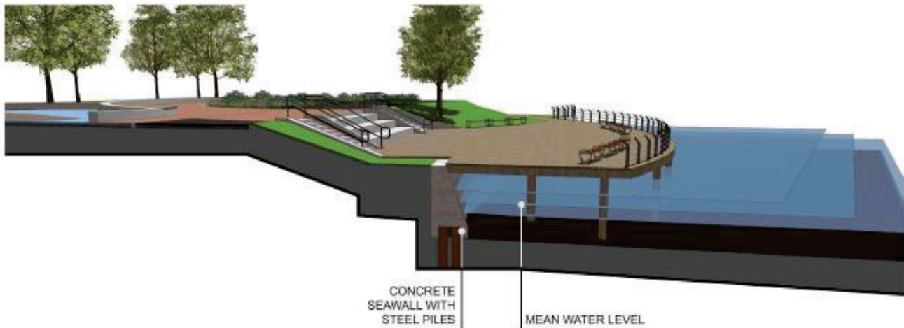
FIGURE 3 Cross-section of the proposed seawall and overlook trail plaza area in Alternative B, Option 2
