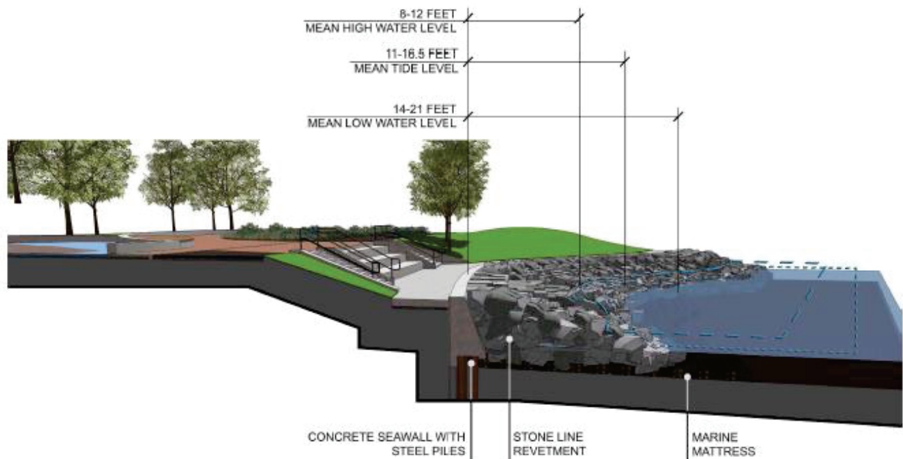
Figure 2 Cross-section of proposed concrete seawall and revetment in Alternative B, Option 1
