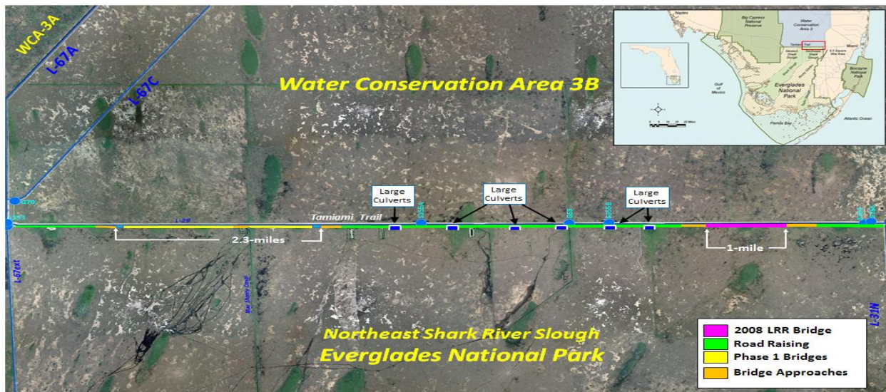
Figure 8. Recommended Phase 2 plan (Alt. 2 from the VA workshop). This plan includes 3.3-miles of bridging, six large culverts, reconstructing the remaining roadway, and replacing the remaining culverts in-kind.
