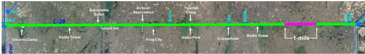
Figure 1A. The Modified Water Deliveries, Tamiami Trail modifications, with the 1-mile bridge (purple) and partial reconstruction of the roadway.
