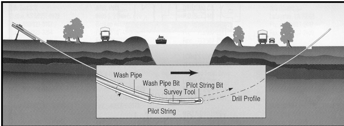
**This schematic shows the process used to install a siphon via HDD. A drill bit is used to drill a hole in a U shape. Reamers are used to gradually make the hole larger until it reaches the appropriate diameter for the proposed pipe. The low point in the pipe needs to be carefully designed and is only applicable in a narrow range of design criteria.**
