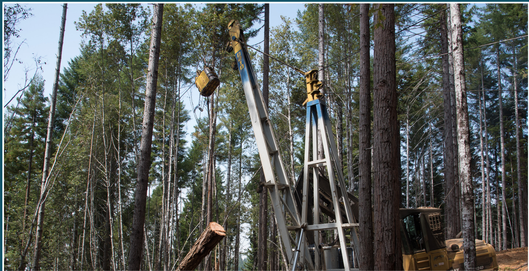
Cable yarding equipment pulls up cut trees on steep slopes to a haul road where they will be removed from the site.
