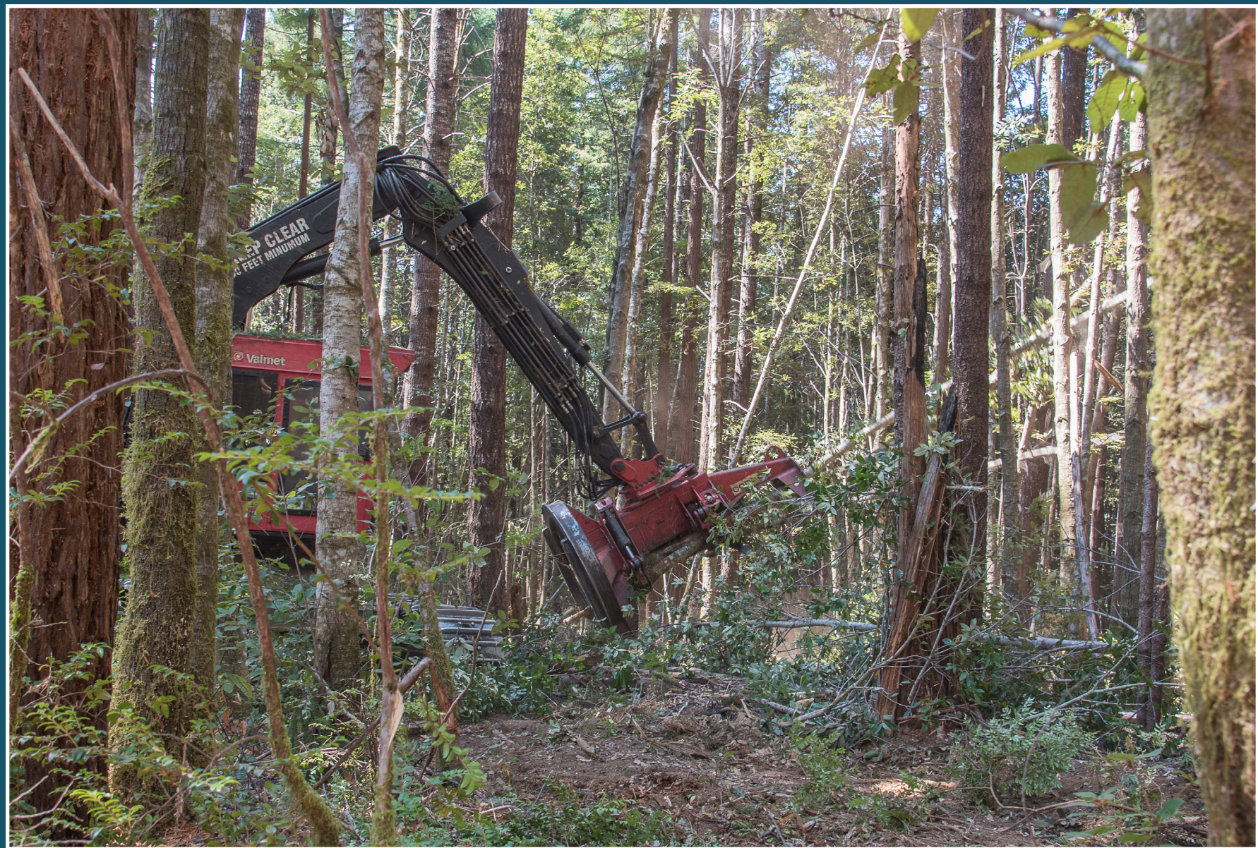
A feller buncher cuts smaller diameter trees as part of a low thin prescription in an ongoing forest restoration project in the upper Lost Man Creek watershed.
