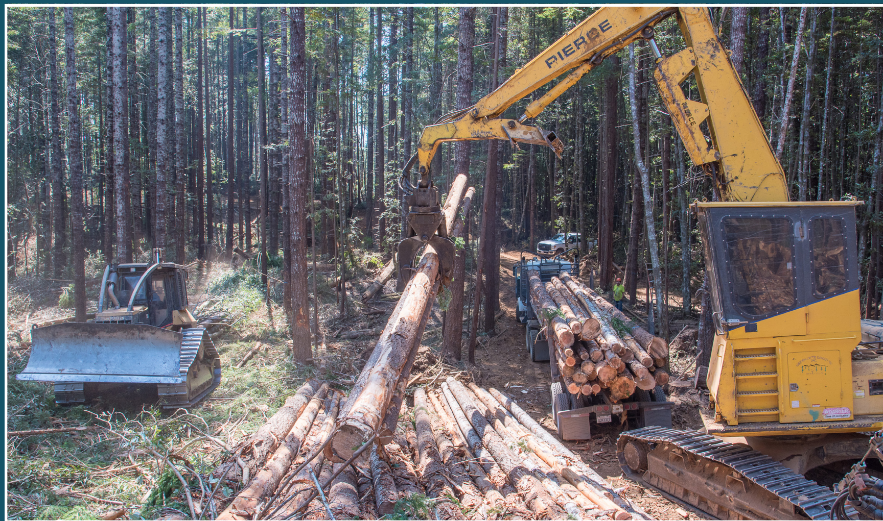
As part of ground-based operations, a skidder pulls cut trees to a small landing, where they are processed and loaded onto a haul truck.
