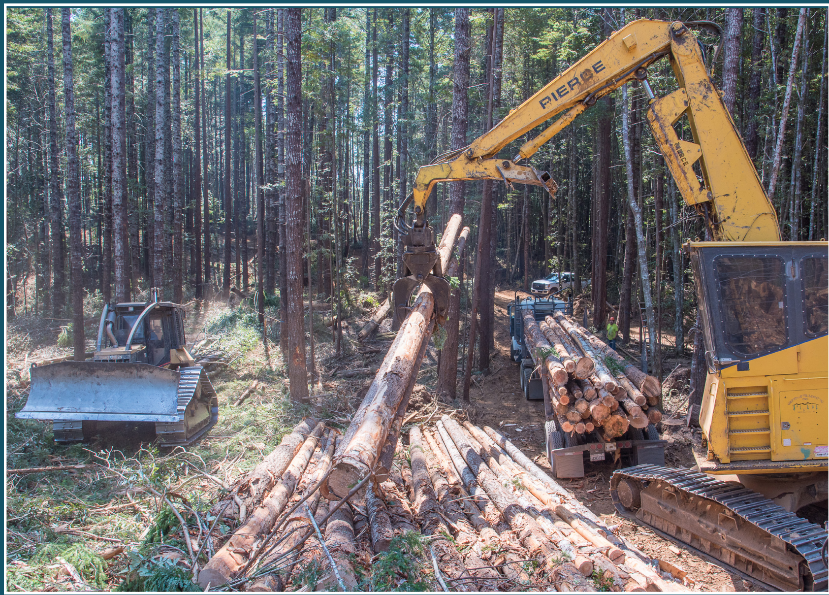
As part of ground-based operations, a skidder pulls cut trees to a small landing where they are processed and loaded onto a haul truck.
