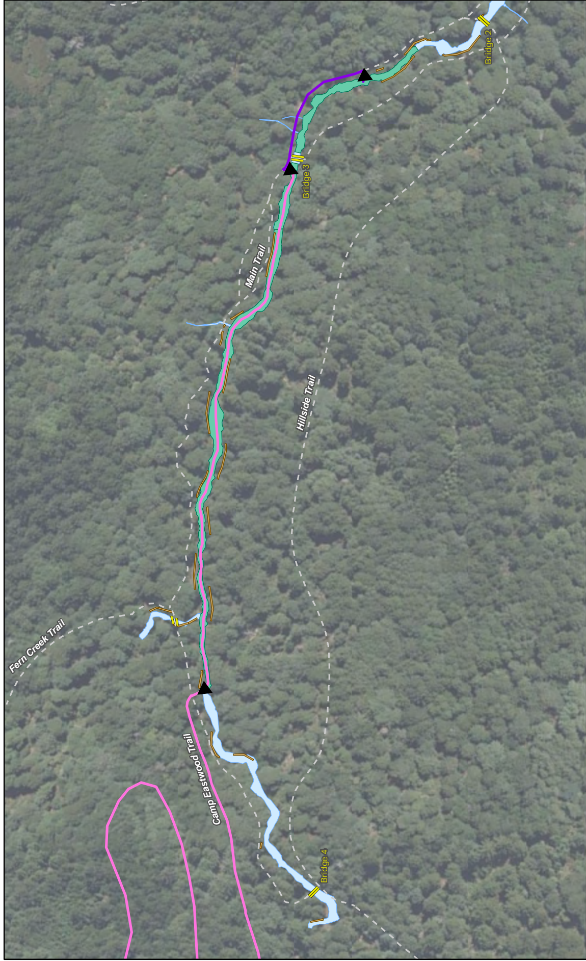
Figure 2-11 Proposed Equipment Access for Riprap Removal Upstream of Bridge 2 Muir Woods National Monument Salmon Habitat Enhancement and Bridge Replacement Project Zone of Dewatering Existing Riprap Location Bridge Primary Route for Large Excavator Route On Trail Trail Ramps 0 95 190 380 Feet
