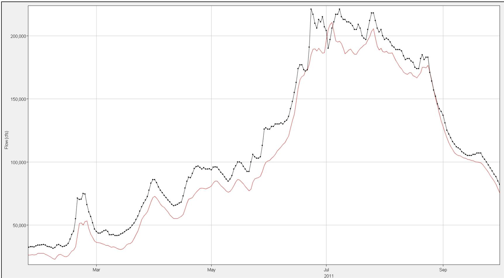
**Figure 8-24: Straddle-Stagger routing results for Omaha-Nebraska City during 2011. Red data are the Straddle-Stagger data and black data are the observed data.**
