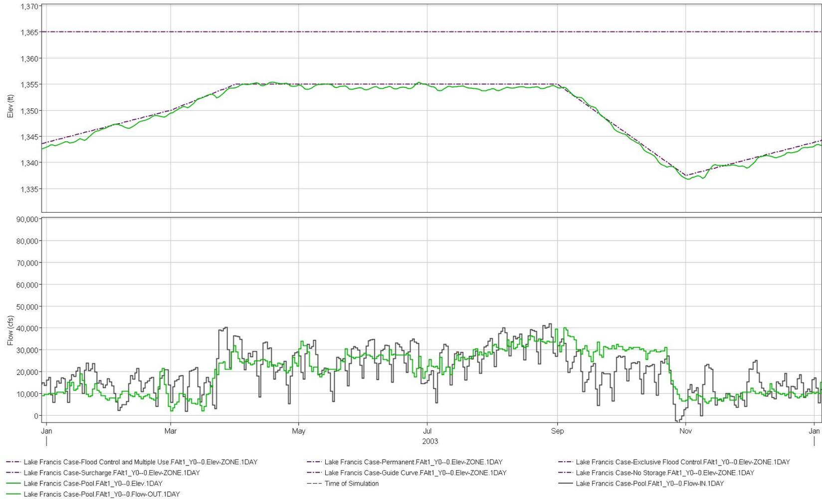
**Figure 5-47: Plot of Fort Randall guide curve operations with a navigation end date of November 1, 1932.**
