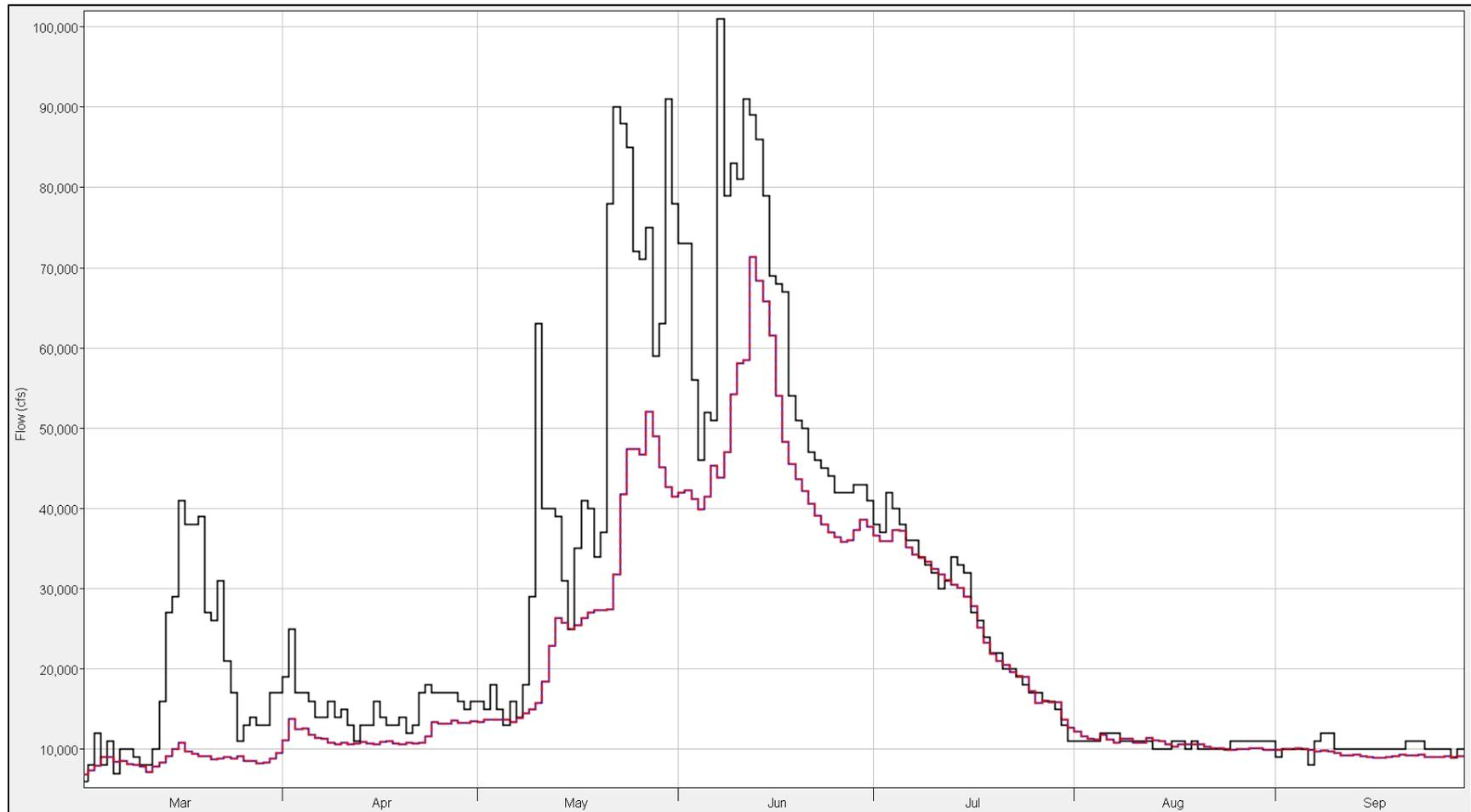
**Figure 8-31: Straddle-Stagger vs. Coefficient routing results for Landusky, MT-Fort Peck during 2011. Red data are the Straddle-Stagger data, blue data are the Coefficient Routing data, and black data are the observed data.**
