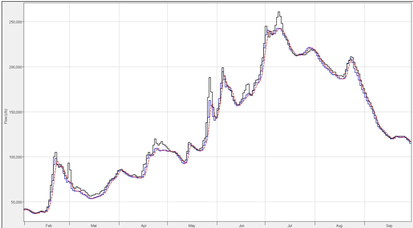
**Figure 8-46: Straddle-Stagger vs. Coefficient routing results for Kansas City-Waverly during 2011. Red data are the Straddle-Stagger data, blue data are the Coefficient Routing data, and black data are the observed data.**
