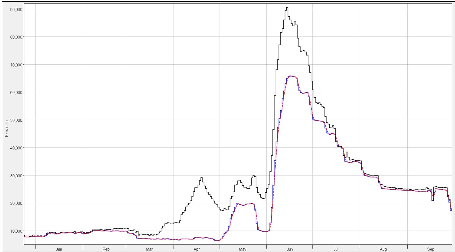
**Figure 8-32: Straddle-Stagger vs. Coefficient routing results for Fort Peck-WPMT during 2011. Red data are the Straddle-Stagger data, blue data are the Coefficient Routing data, and black data are the observed data.**
