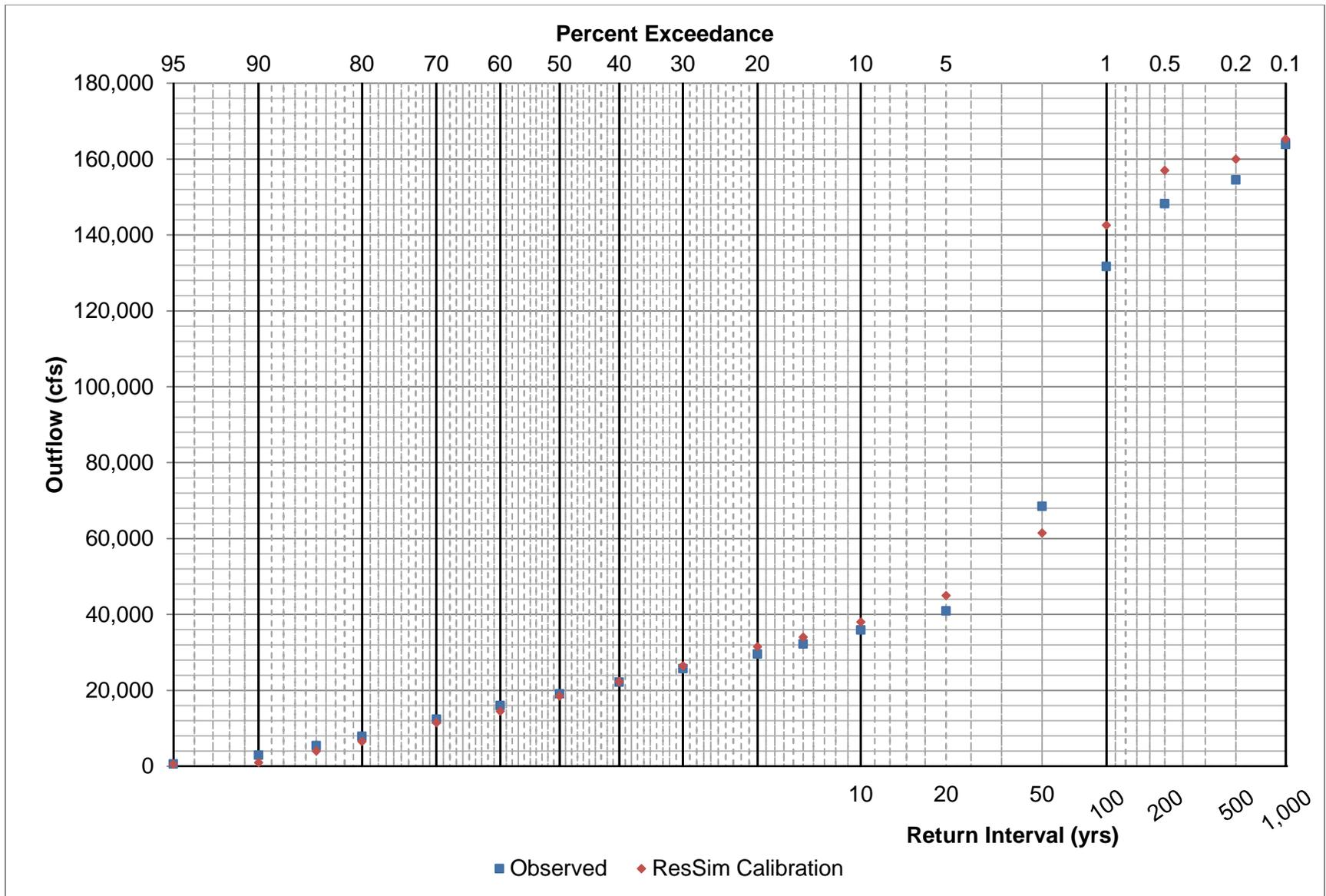
Figure 5-16: Lake Sharpe release probability curves for years 1998-2012.
