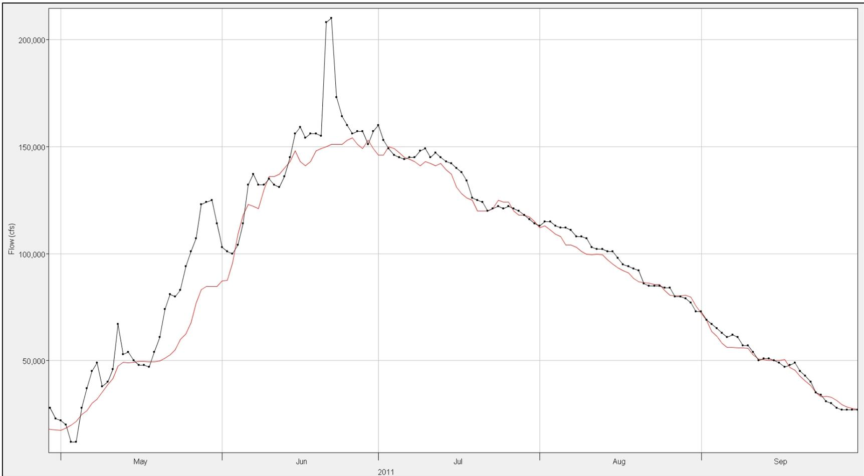
**Figure 8-18: Straddle-Stagger routing results for BIS-Oahe during 2011. Red data are the Straddle-Stagger data and black data are the observed data.**
