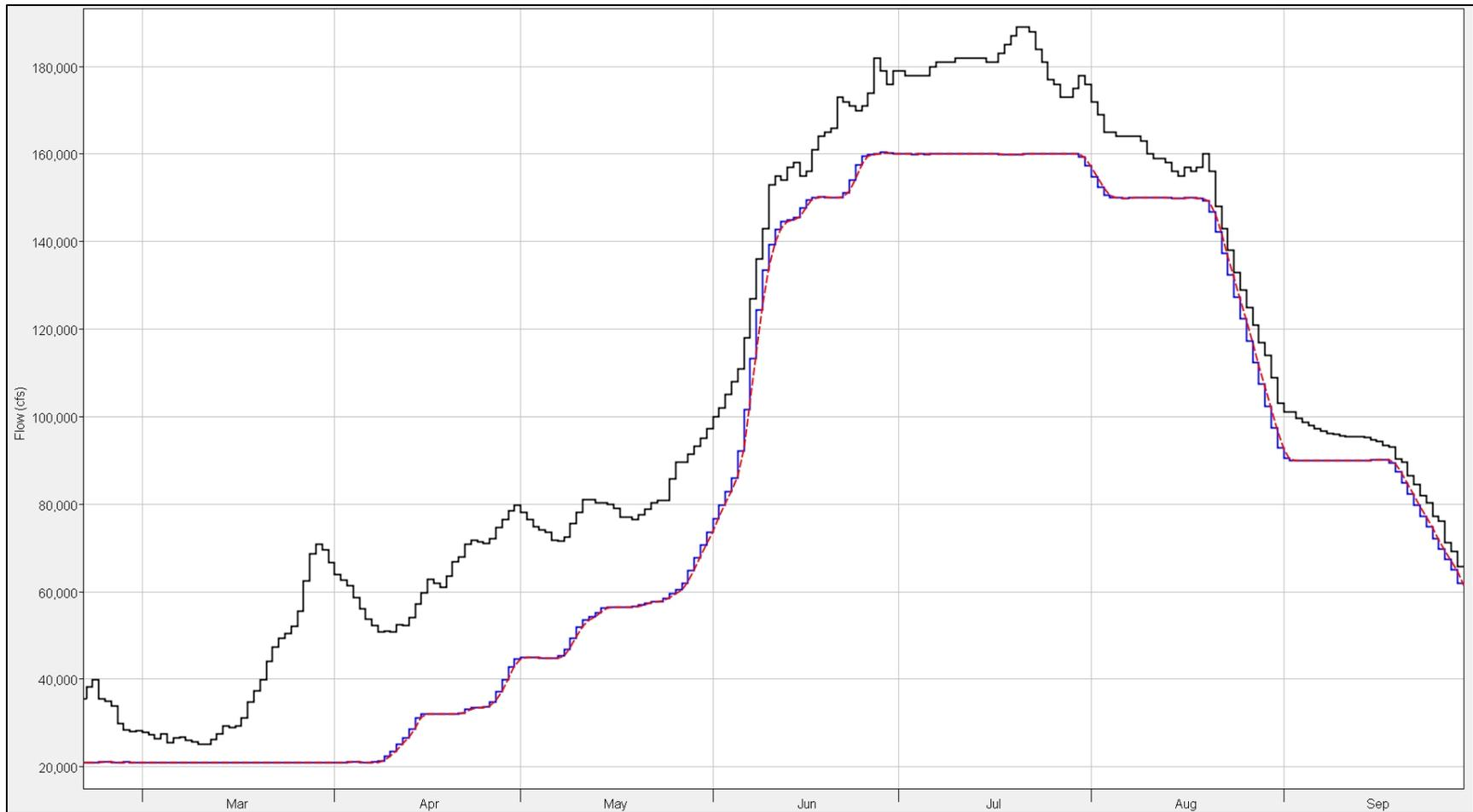
**Figure 8-40: Straddle-Stagger vs. Coefficient routing results for Gavins Point-Sioux City during 2011. Red data are the Straddle-Stagger data, blue data are the Coefficient Routing data, and black data are the observed data.**
