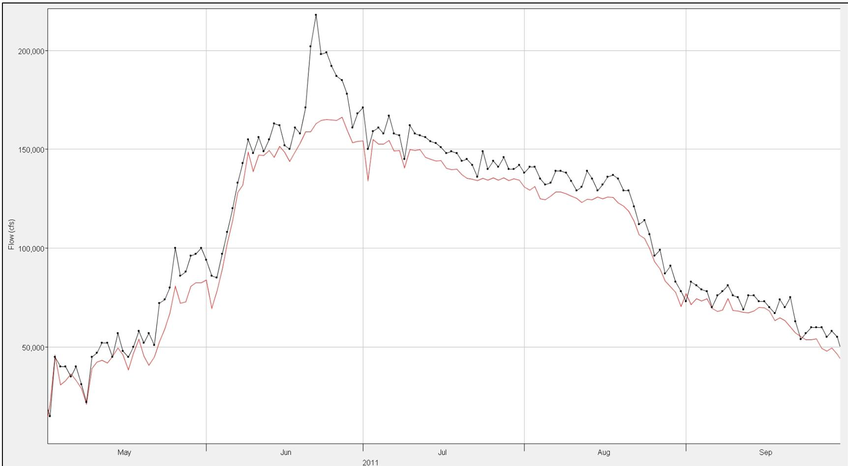
**Figure 8-20: Straddle-Stagger routing results for Big Bend-Fort Randall during 2011. Red data are the Straddle-Stagger data and black data are the observed data.**
