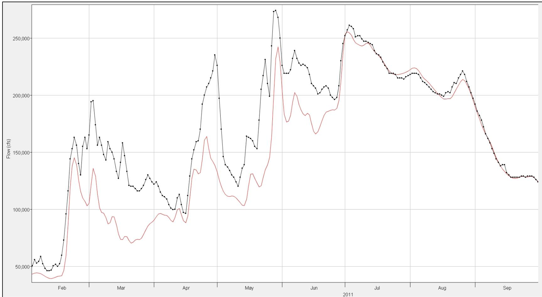
**Figure 8-30: Straddle-Stagger routing results for Boonville-Hermann during 2011. Red data are the Straddle-Stagger data and black data are the observed data.**
