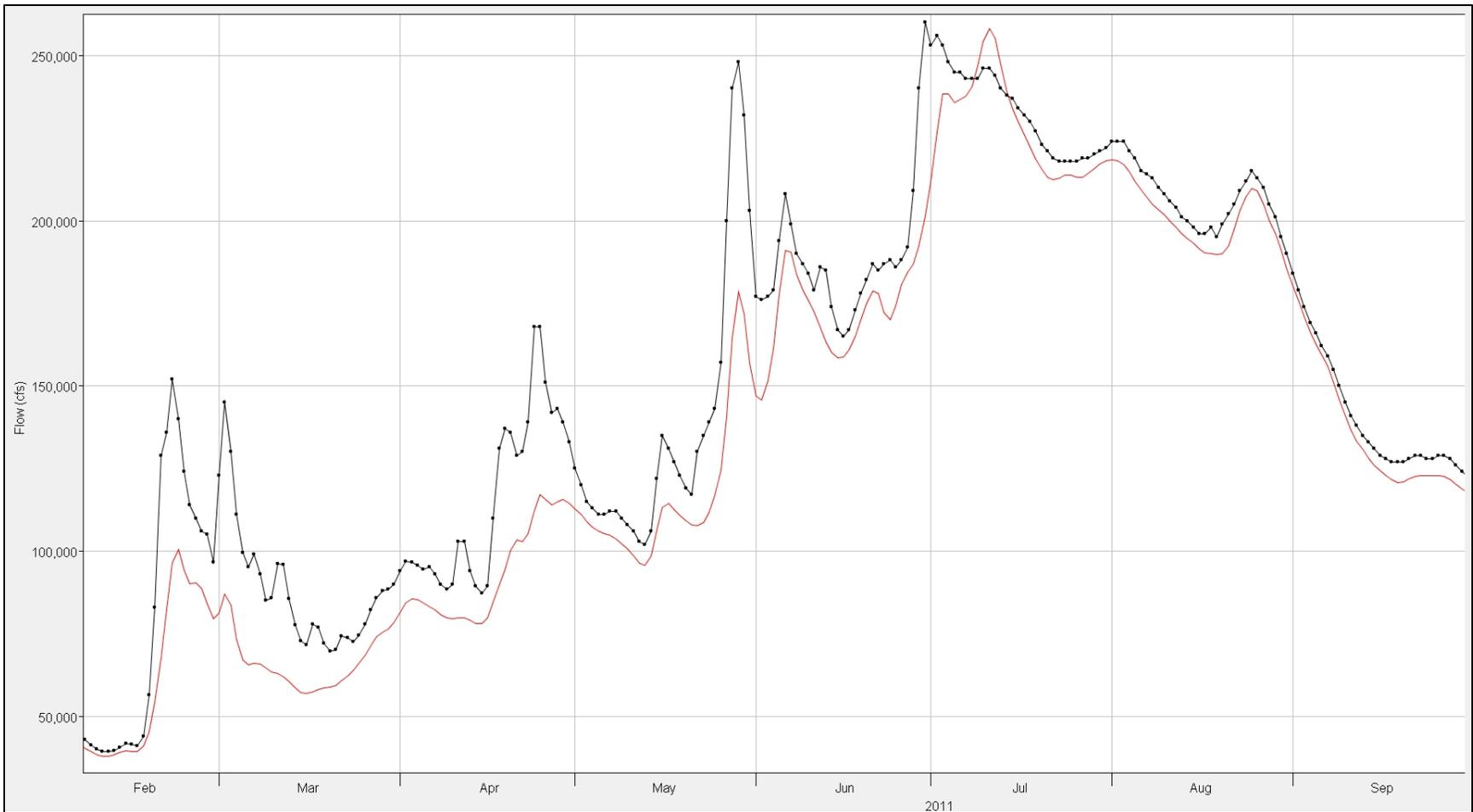
**Figure 8-29: Straddle-Stagger routing results for Waverly-Boonville during 2011. Red data are the Straddle-Stagger data and black data are the observed data.**
