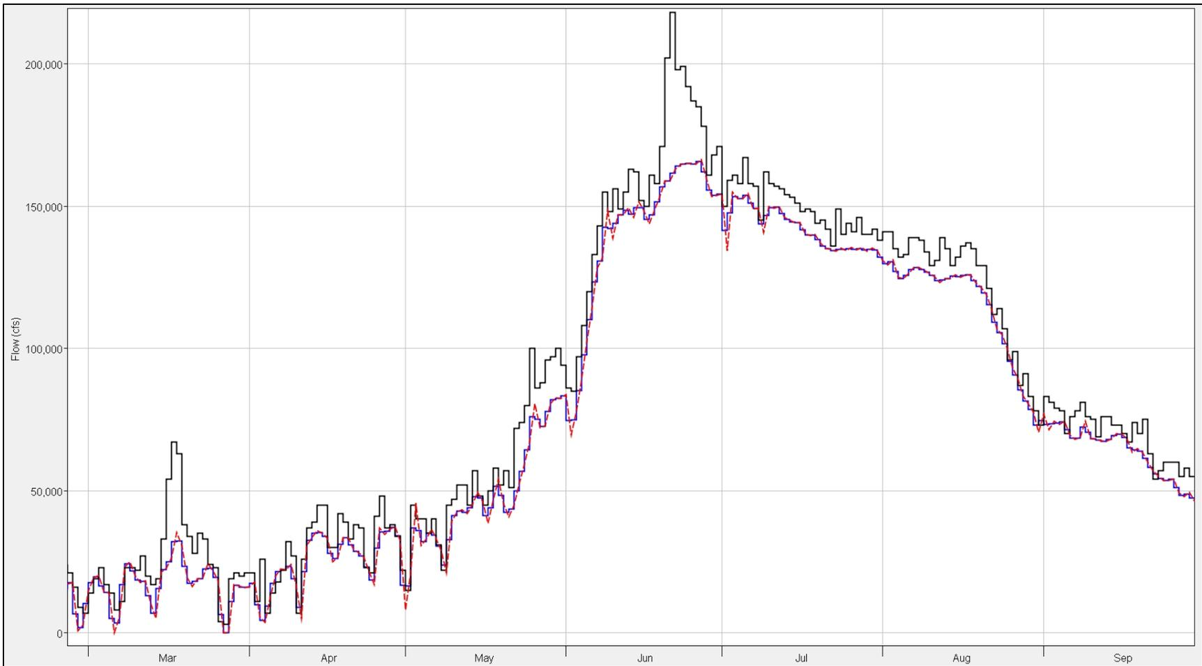
**Figure 8-38: Straddle-Stagger vs. Coefficient routing results for Big Bend-Fort Randall during 2011. Red data are the Straddle-Stagger data, blue data are the Coefficient Routing data, and black data are the observed data.**
