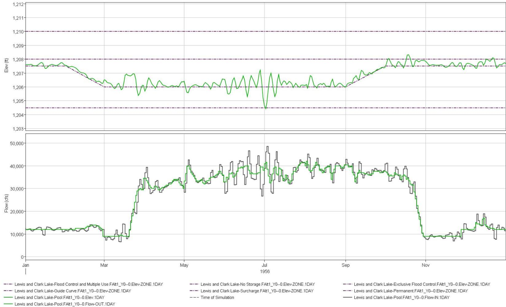
**Figure 5-48: Plot of Gavins Point's guide curve operations in 1956.**
