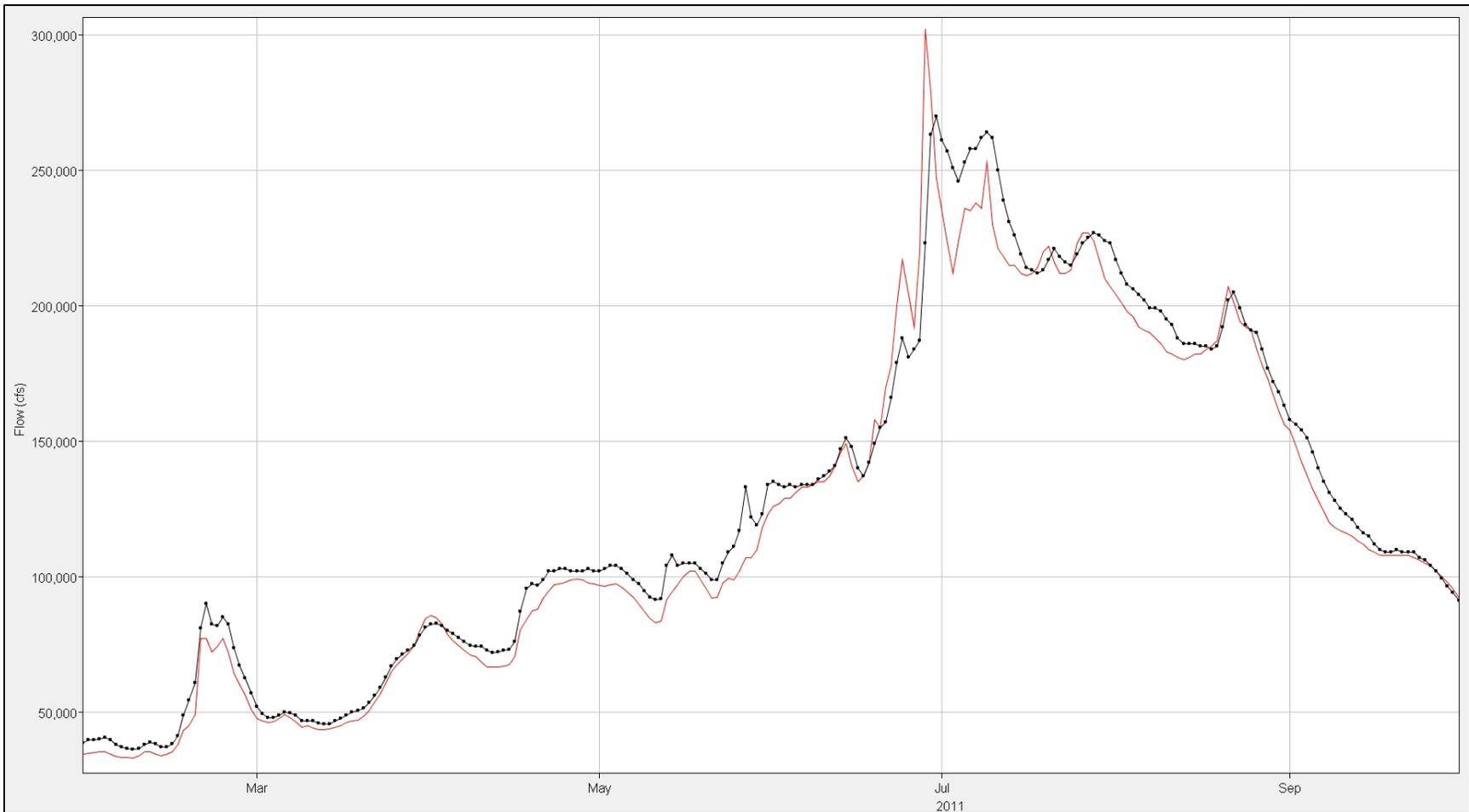
**Figure 8-26: Straddle-Stagger routing results for Rulo-St. Joseph during 2011. Red data are the Straddle-Stagger data and black data are the observed data.**
