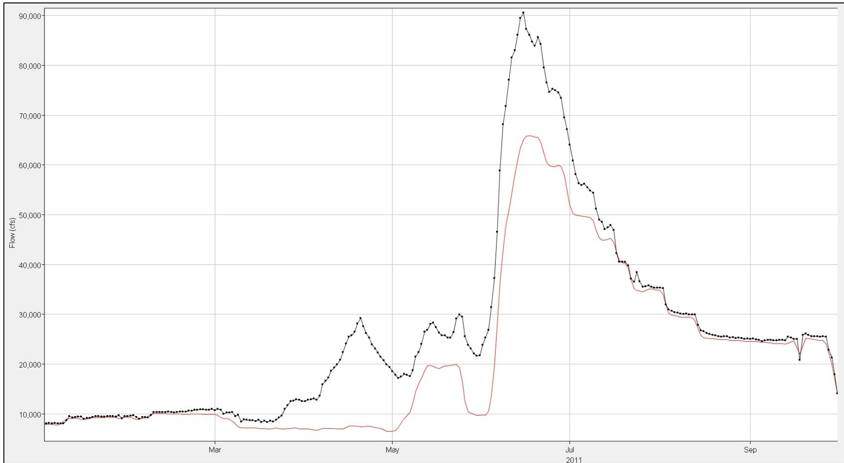
**Figure 8-14: Straddle-Stagger routing results for Fort Peck-WPMT during 2011. Red data are the Straddle-Stagger data and black data are the observed data.**
