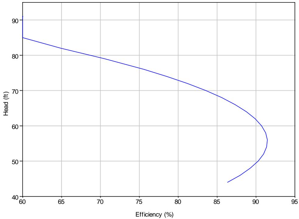
**Figure 3-36: Big Bend powerplant efficiency.**
