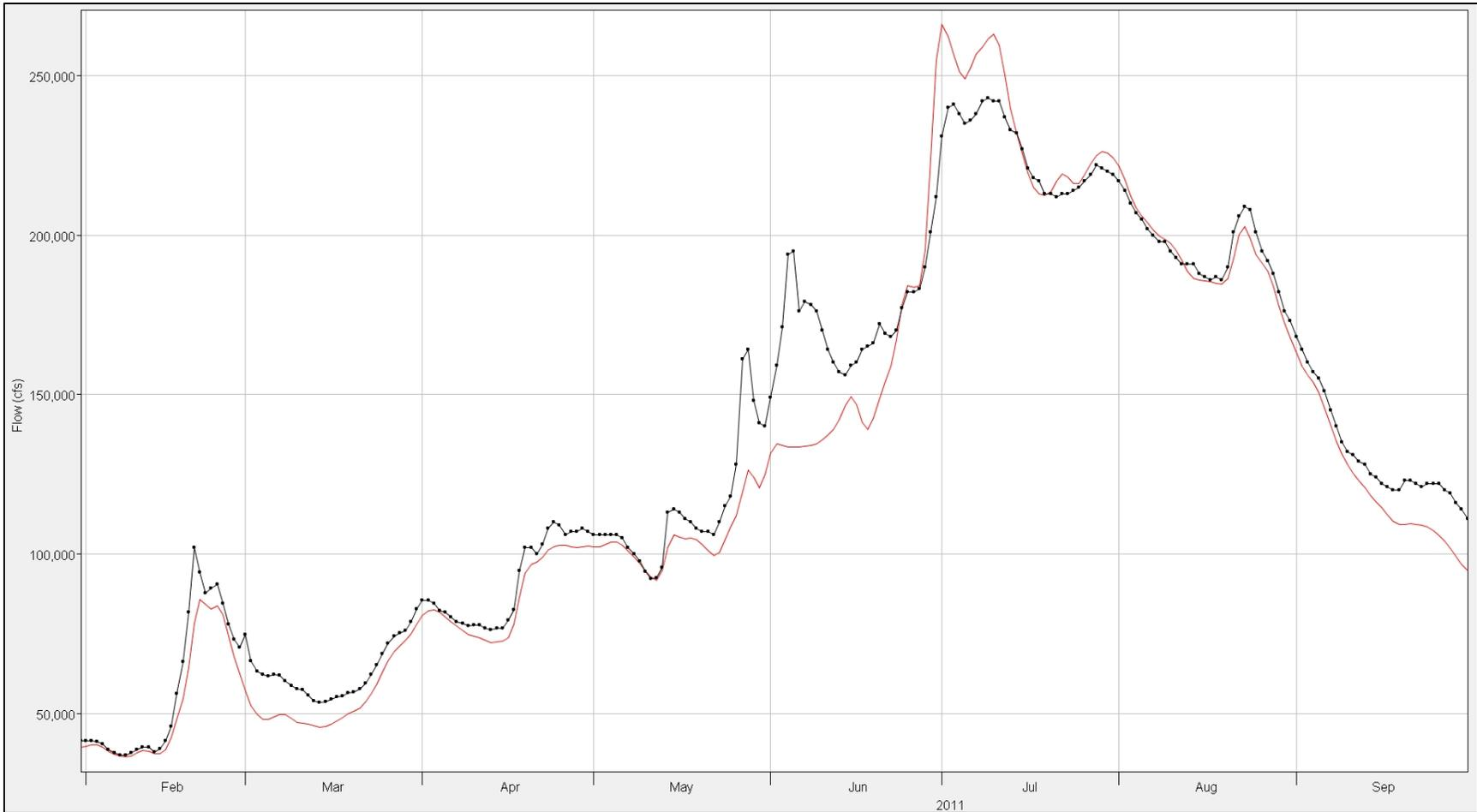
**Figure 8-27: Straddle-Stagger routing results for St. Joseph-Kansas City during 2011. Red data are the Straddle-Stagger data and black data are the observed data.**
