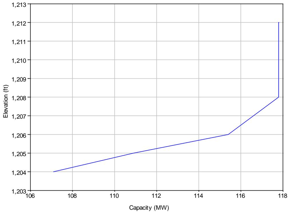
**Figure 3-26: Gavins Point power generation capacity.**
