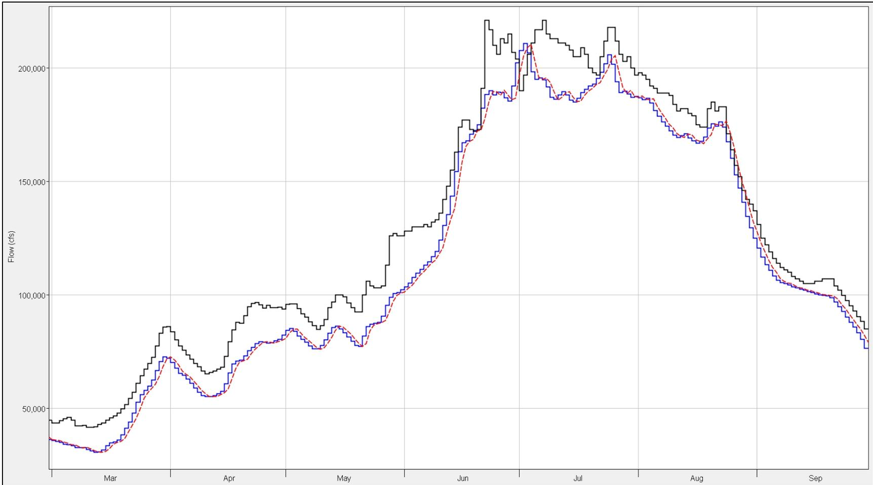
**Figure 8-42: Straddle-Stagger vs. Coefficient routing results for Omaha-Nebraska City during 2011. Red data are the Straddle-Stagger data, blue data are the Coefficient Routing data, and black data are the observed data.**
