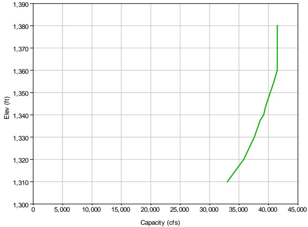
**Figure 3-19: FTRA powerhouse discharge capacity.**
