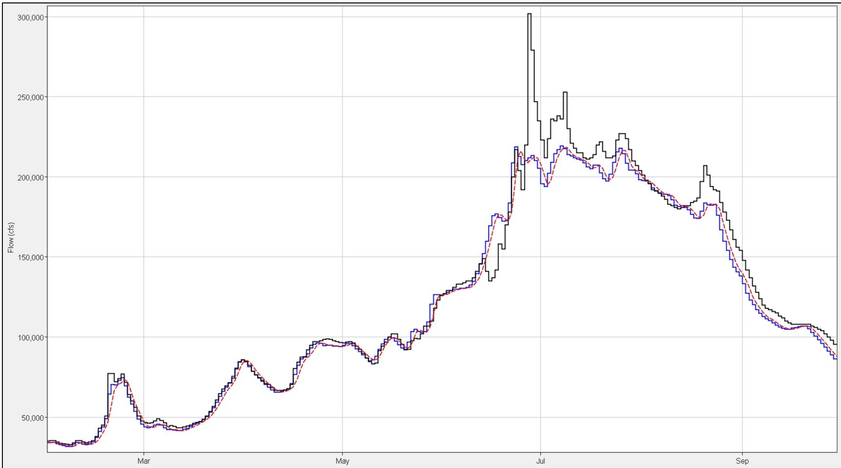
**Figure 8-43: Straddle-Stagger vs. Coefficient routing results for Nebraska City-Rulo during 2011. Red data are the Straddle-Stagger data, blue data are the Coefficient Routing data, and black data are the observed data.**
