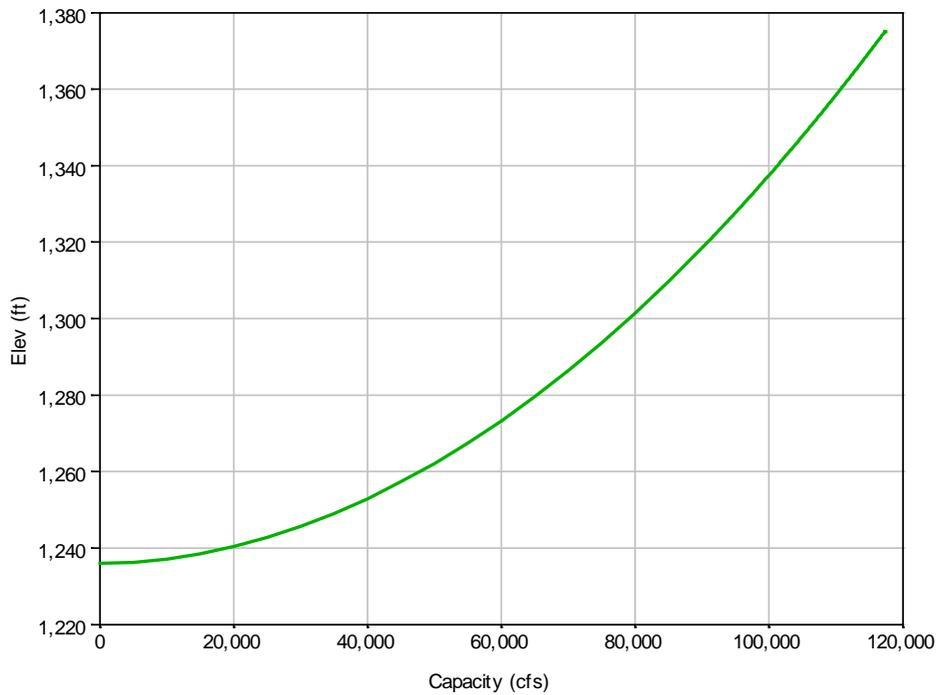
**Figure 3-15: Fort Randall outlet works capacity curve.**
