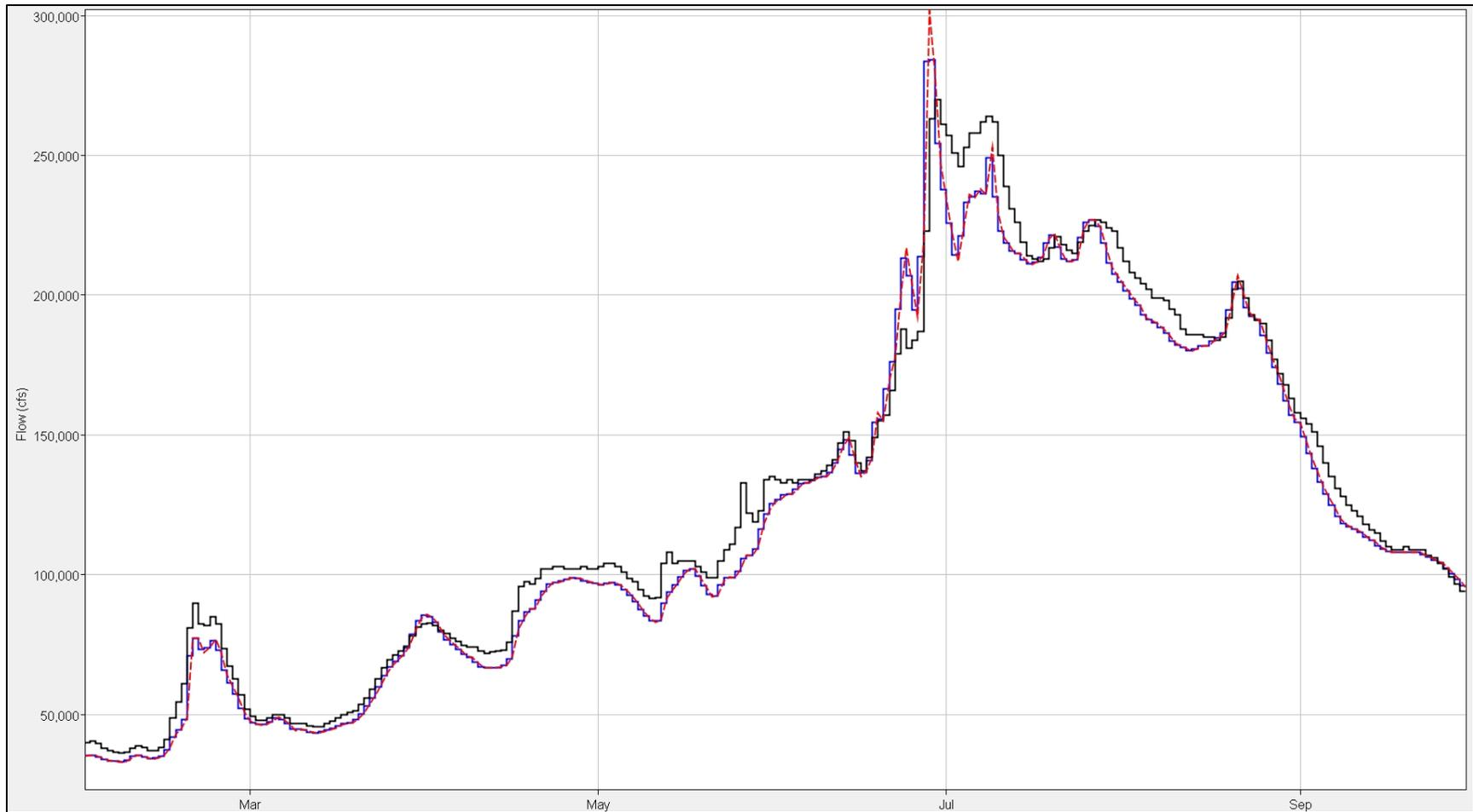
**Figure 8-44: Straddle-Stagger vs. Coefficient routing results for Rulo-St. Joseph during 2011. Red data are the Straddle-Stagger data, blue data are the Coefficient Routing data, and black data are the observed data.**
