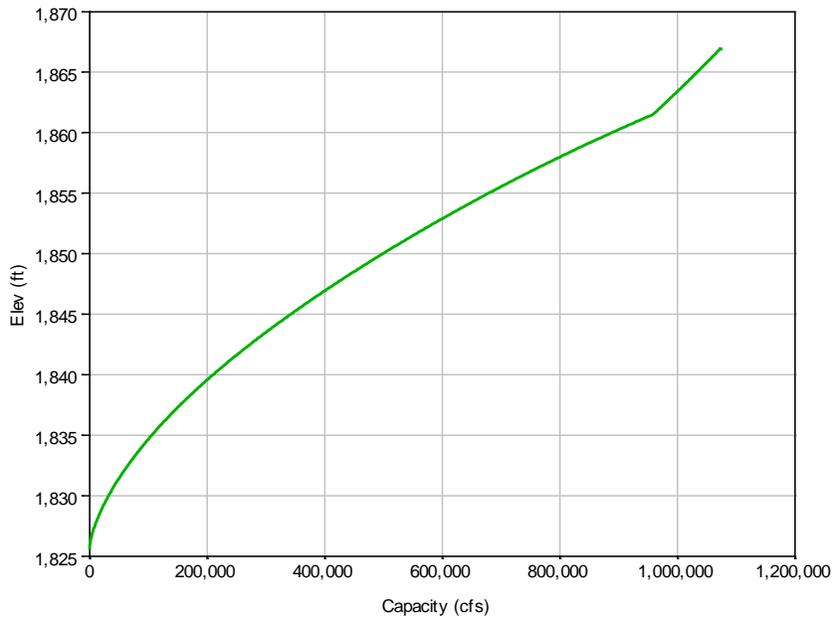
**Figure 3-8: Garrison spillway capacity curve.**
