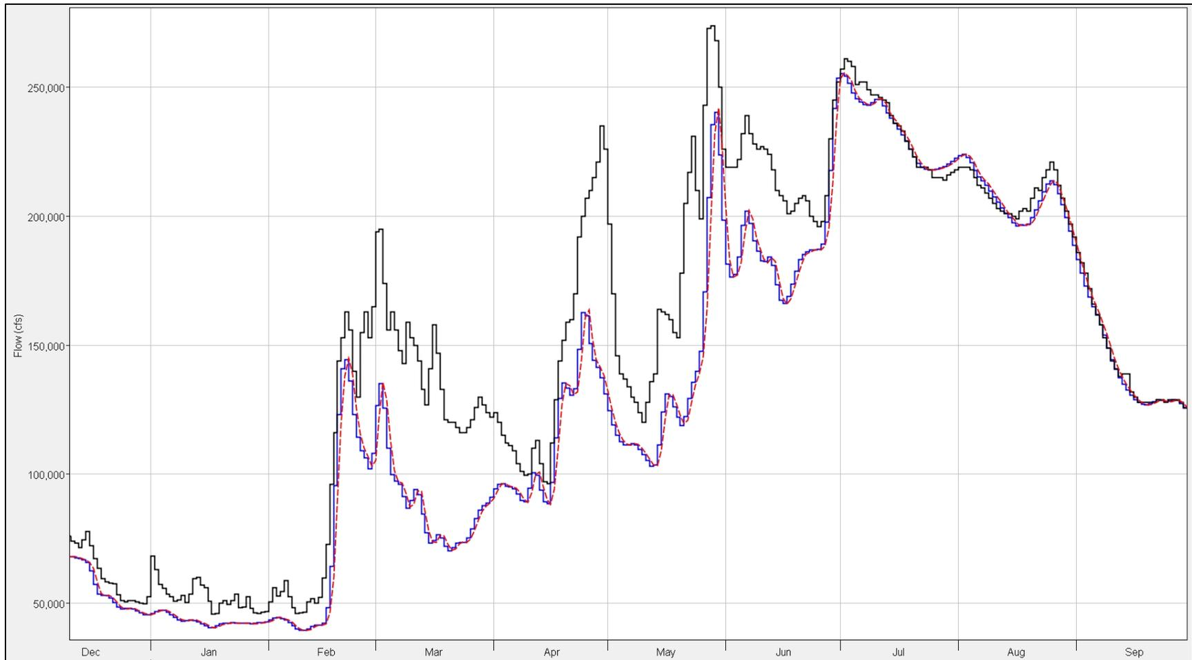
**Figure 8-48: Straddle-Stagger vs. Coefficient routing results for Boonville-Hermann during 2011. Red data are the Straddle-Stagger data, blue data are the Coefficient Routing data, and black data are the observed data.**
