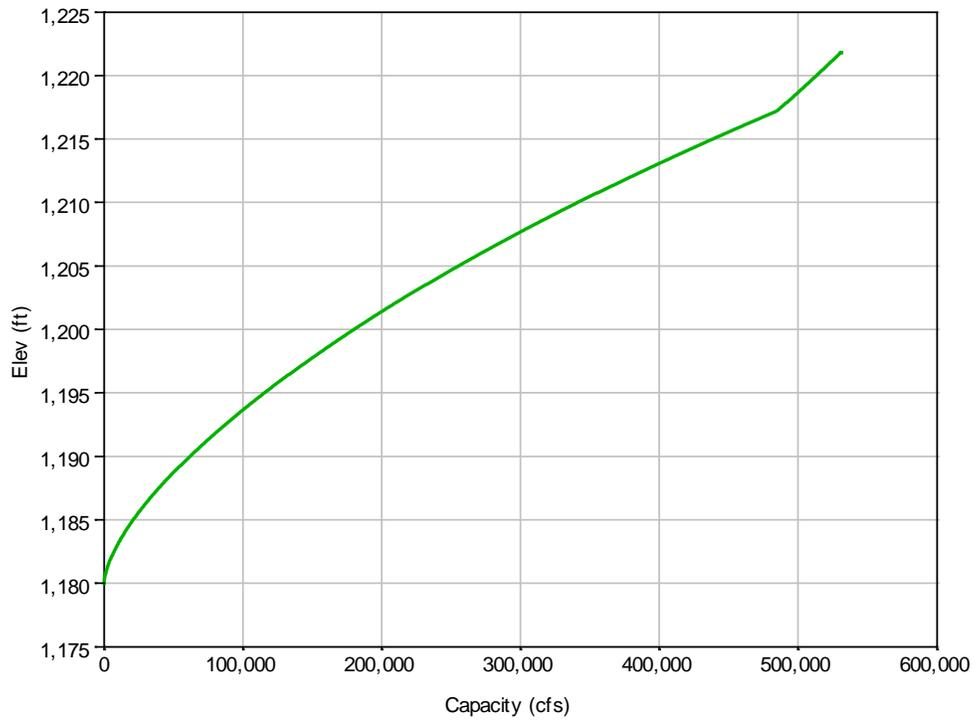
**Figure 3-12: Gavins Point spillway capacity curve.**
