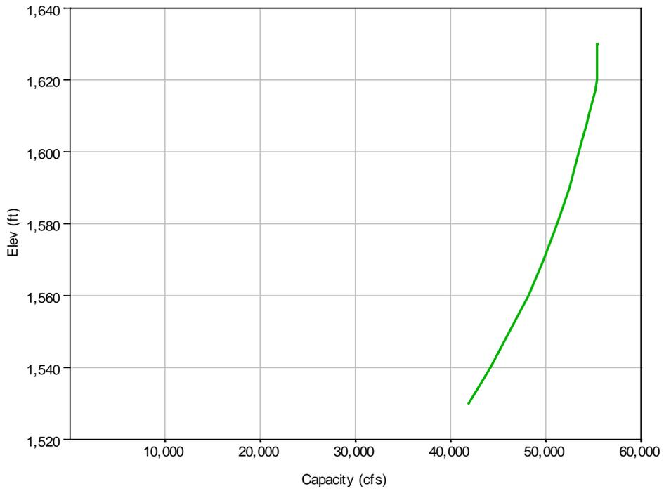
**Figure 3-18: Oahe powerhouse discharge capacity.**
