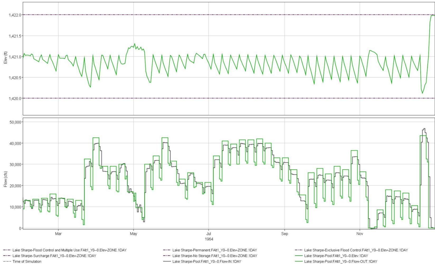
**Figure 5-45: Plot of Big Bend guide curve operations in 1964.**
