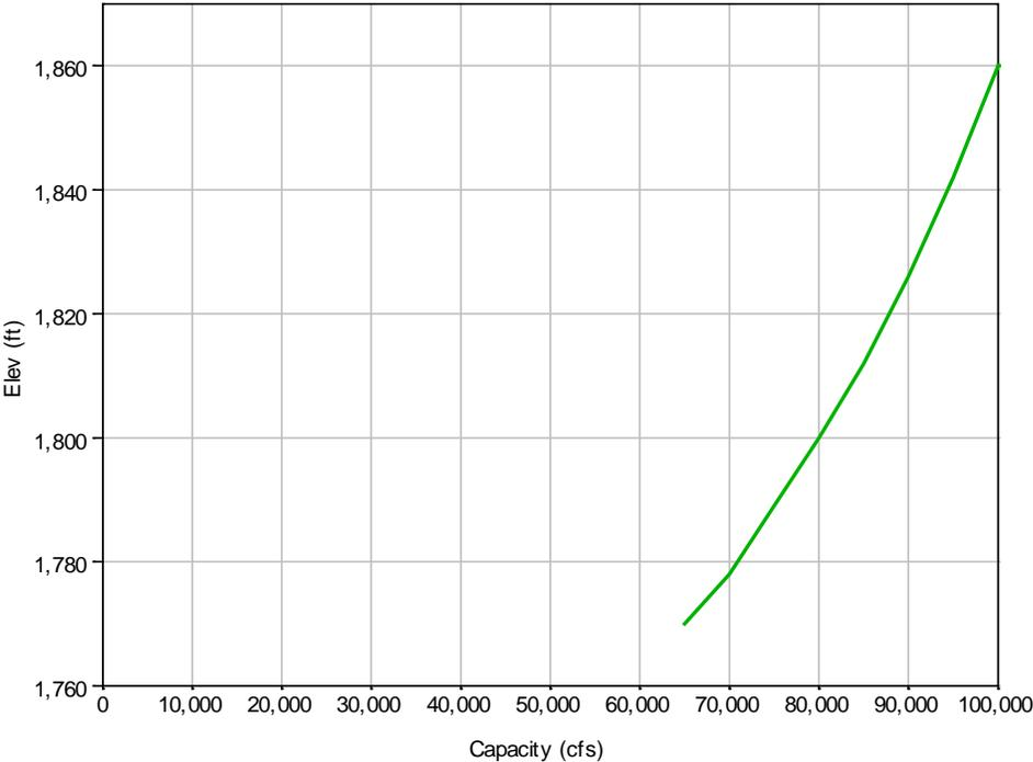
**Figure 3-13: Garrison outlet works capacity curve.**
