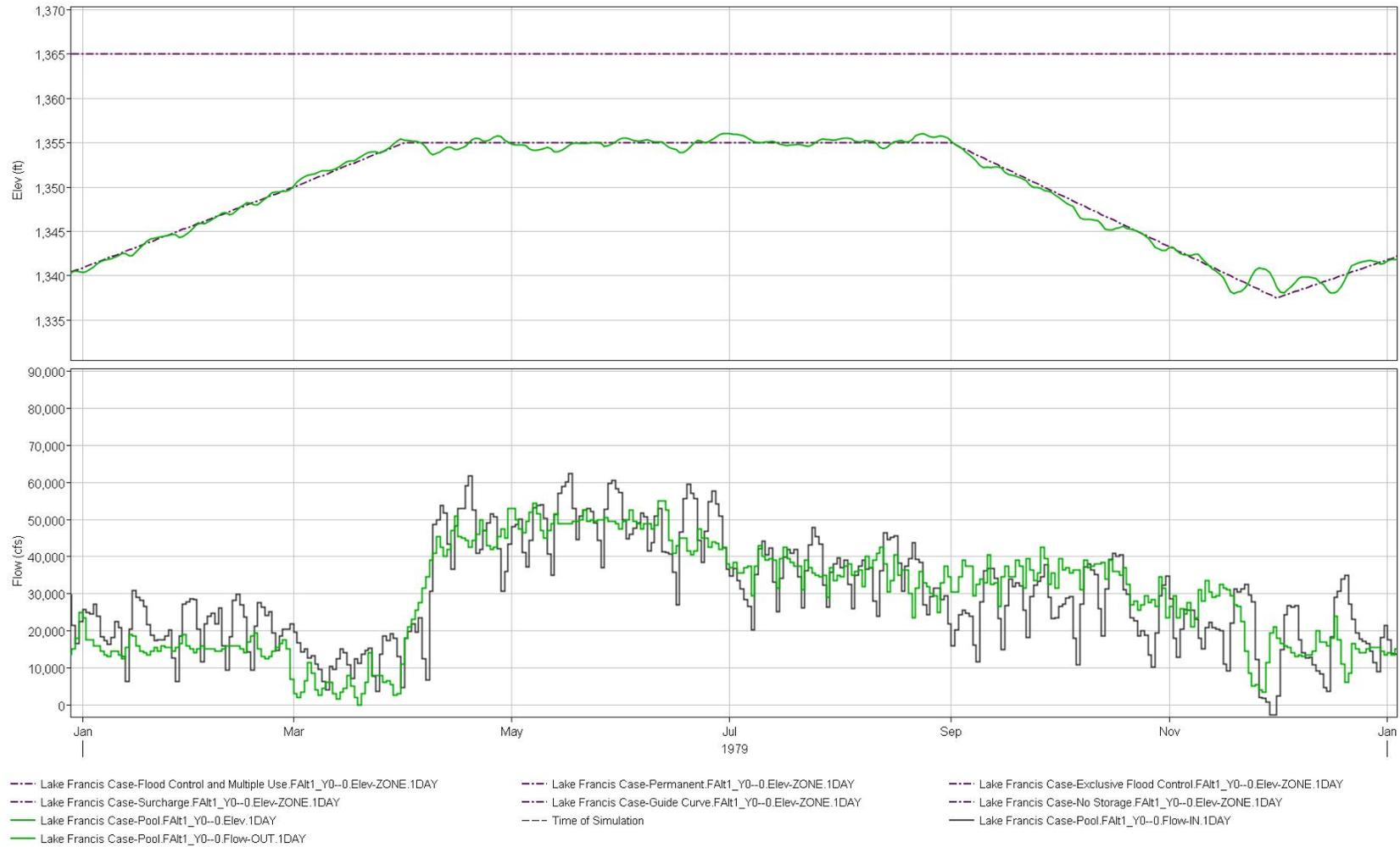
**Figure 5-46: Plot of Fort Randall guide curve operations with a navigation end date of December 1, 1979.**
