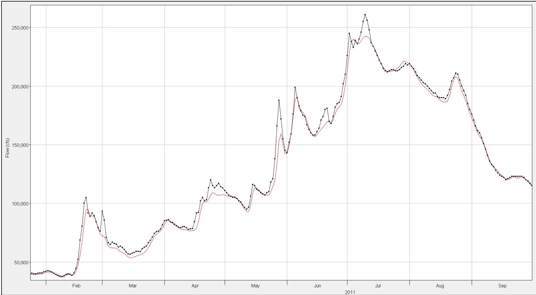
**Figure 8-28: Straddle-Stagger routing results for Kansas City-Waverly during 2011. Red data are the Straddle-Stagger data and black data are the observed data.**
