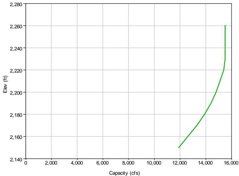
Figure 3-16: Fort Peck powerhouse discharge capacity.
