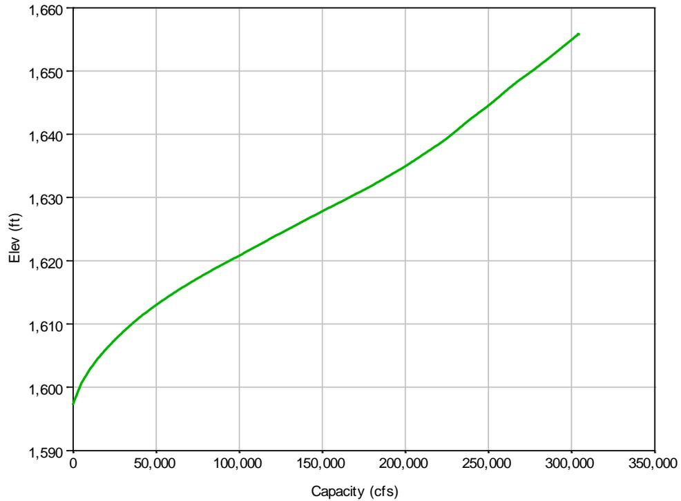
**Figure 3-9: Oahe spillway capacity curve.**
