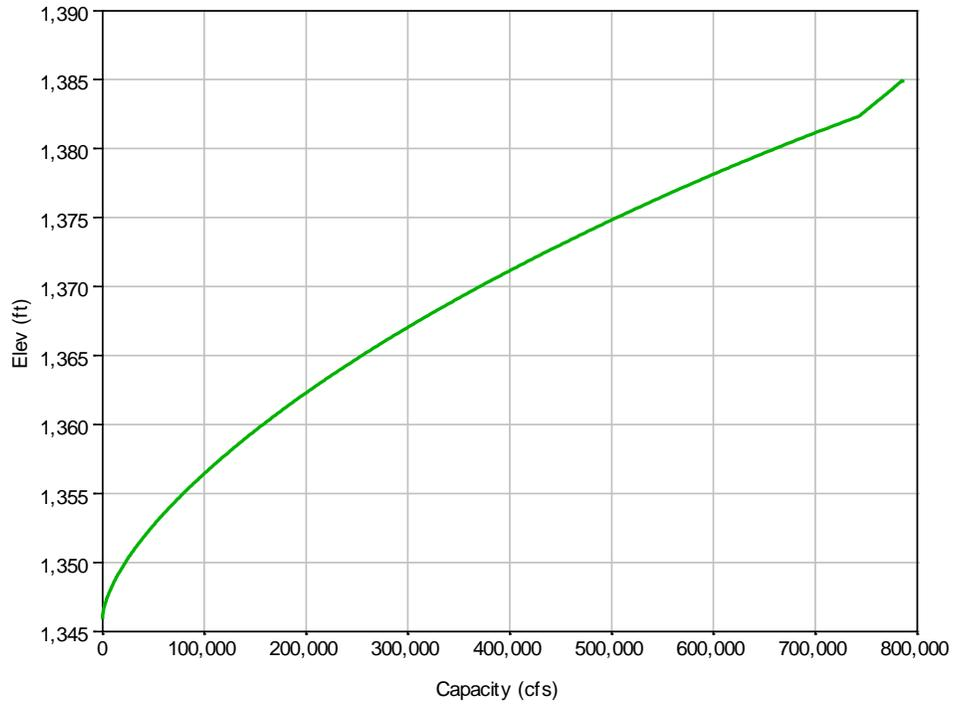
**Figure 3-11: FTRA spillway capacity curve.**
