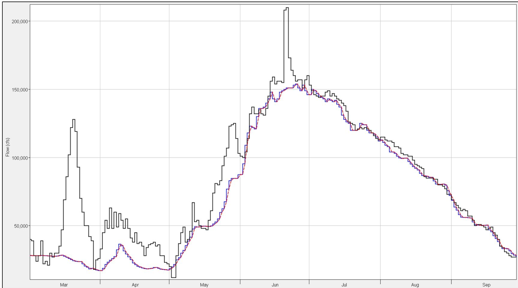
**Figure 8-36: Straddle-Stagger vs. Coefficient routing results for BIS-Oahe during 2011. Red data are the Straddle-Stagger data, blue data are the Coefficient Routing data, and black data are the observed data.**
