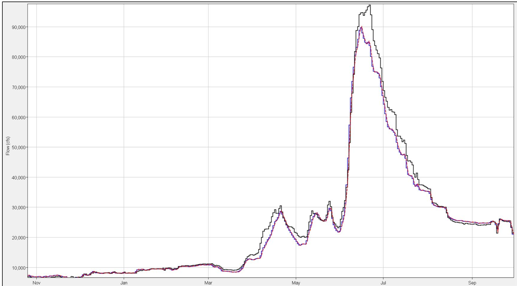
**Figure 8-33: Straddle-Stagger vs. Coefficient routing results for WPMT-CLMT during 2011. Red data are the Straddle-Stagger data, blue data are the Coefficient Routing data, and black data are the observed data.**
