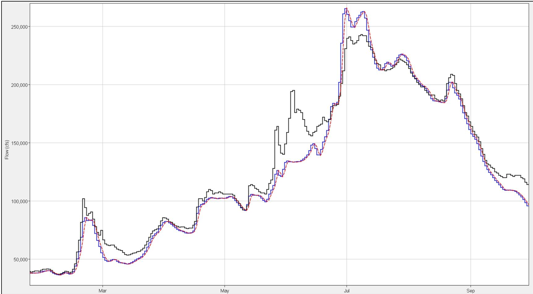
**Figure 8-45: Straddle-Stagger vs. Coefficient routing results for St. Joseph-Kansas City during 2011. Red data are the Straddle-Stagger data, blue data are the Coefficient Routing data, and black data are the observed data.**
