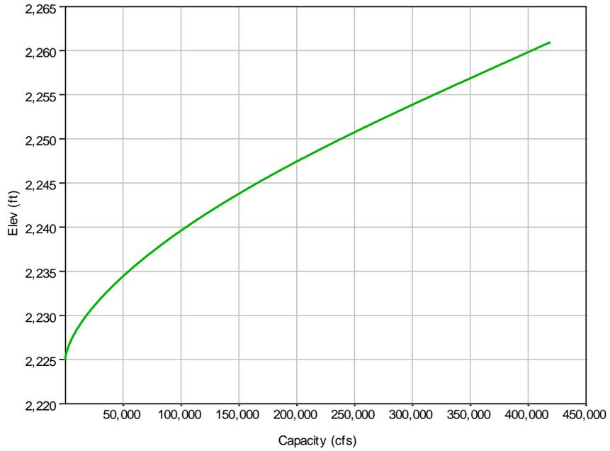
**Figure 3-7: Fort Peck spillway capacity curve.**
