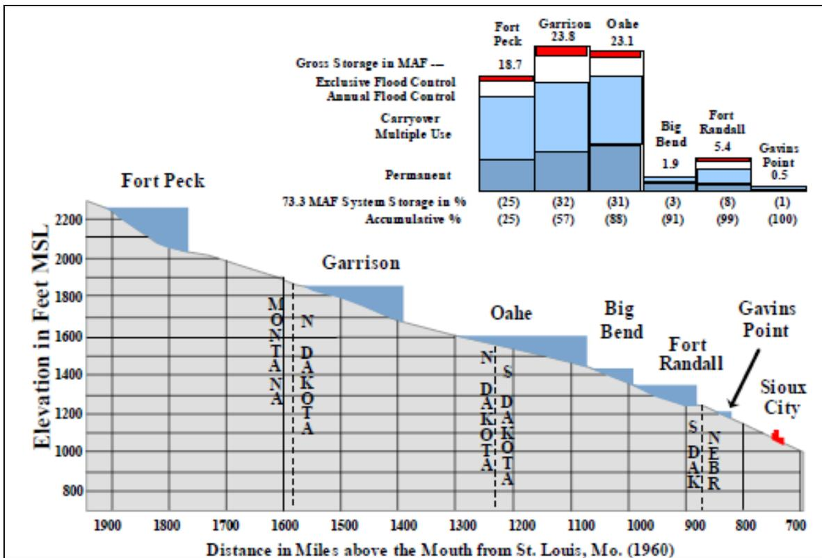
**Figure 2-4: Profile of mainstem System and storage capacities**
