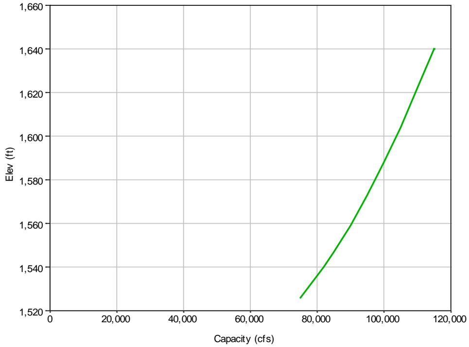
**Figure 3-14: Oahe outlet works capacity curve.**
