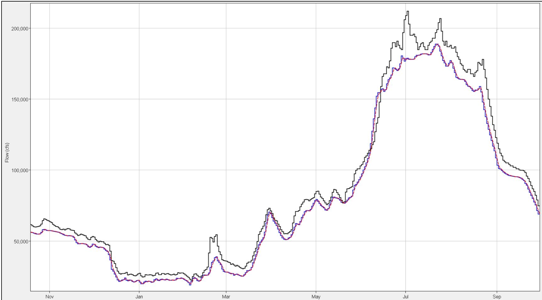
**Figure 8-41: Straddle-Stagger vs. Coefficient routing results for Sioux City-Omaha during 2011. Red data are the Straddle-Stagger data, blue data are the Coefficient Routing data, and black data are the observed data.**
