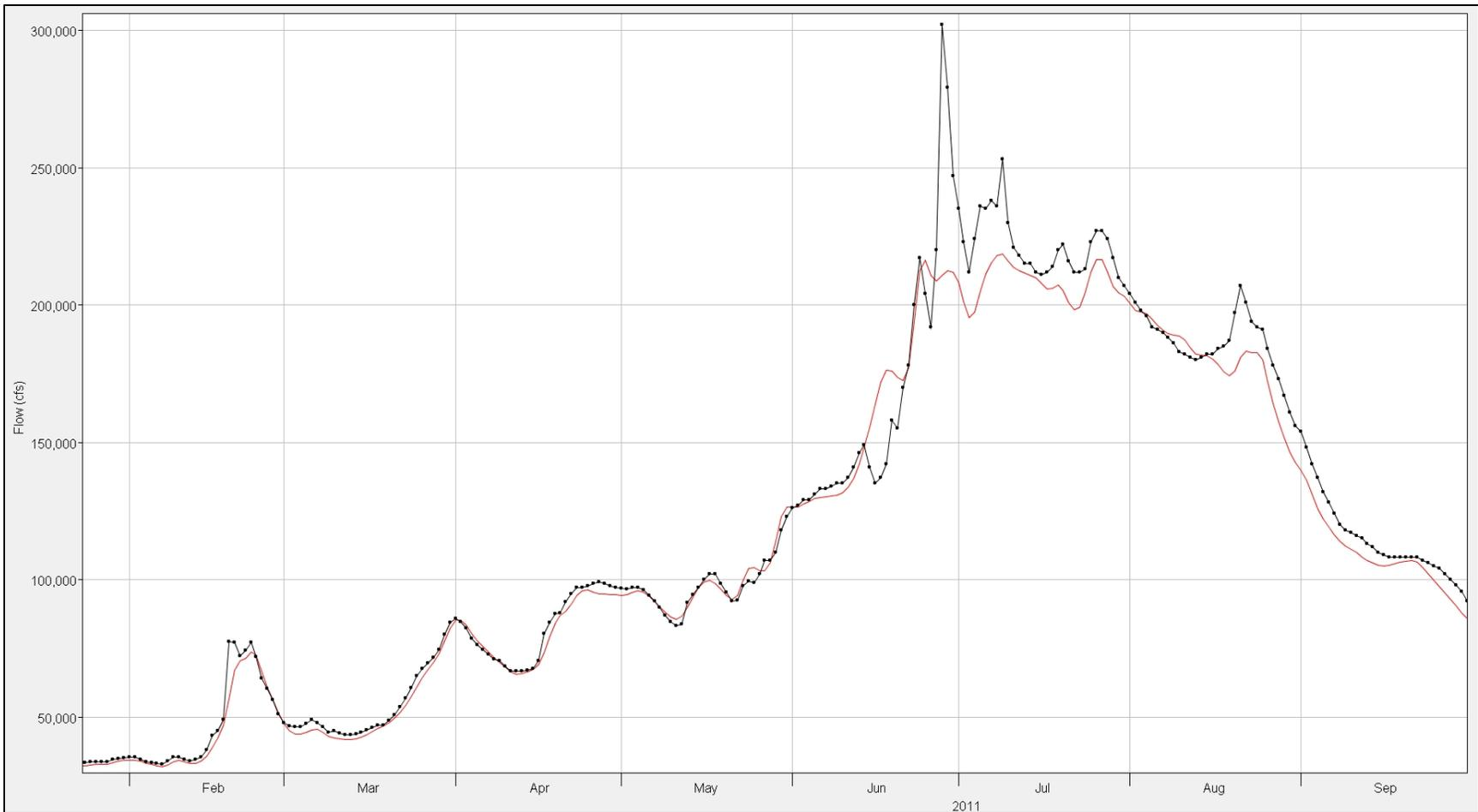
**Figure 8-25: Straddle-Stagger routing results for Nebraska City-Rulo during 2011. Red data are the Straddle-Stagger data and black data are the observed data.**
