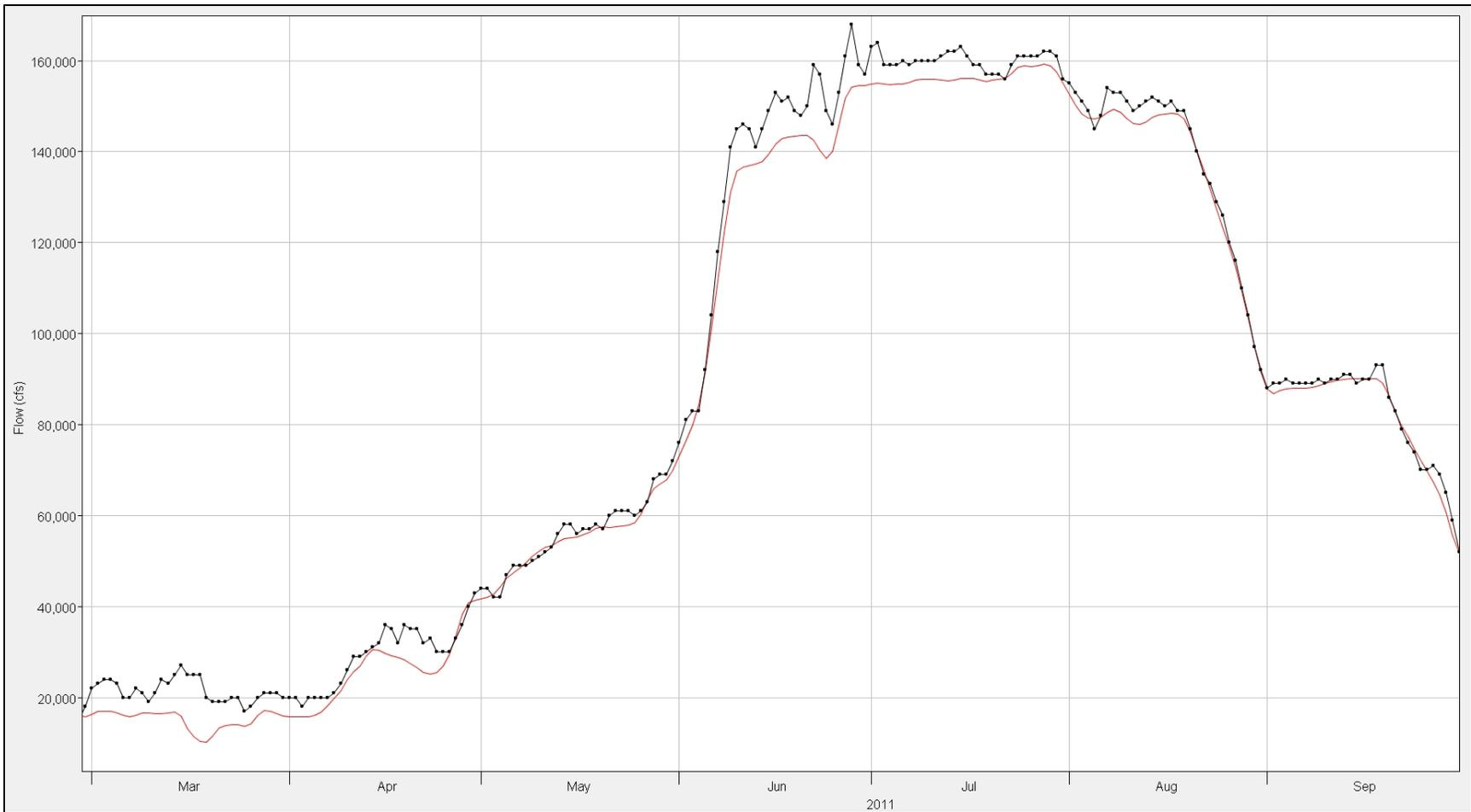
**Figure 8-21: Straddle-Stagger routing results for Fort Randall-Gavins Point during 2011. Red data are the Straddle-Stagger data and black data are the observed data.**
