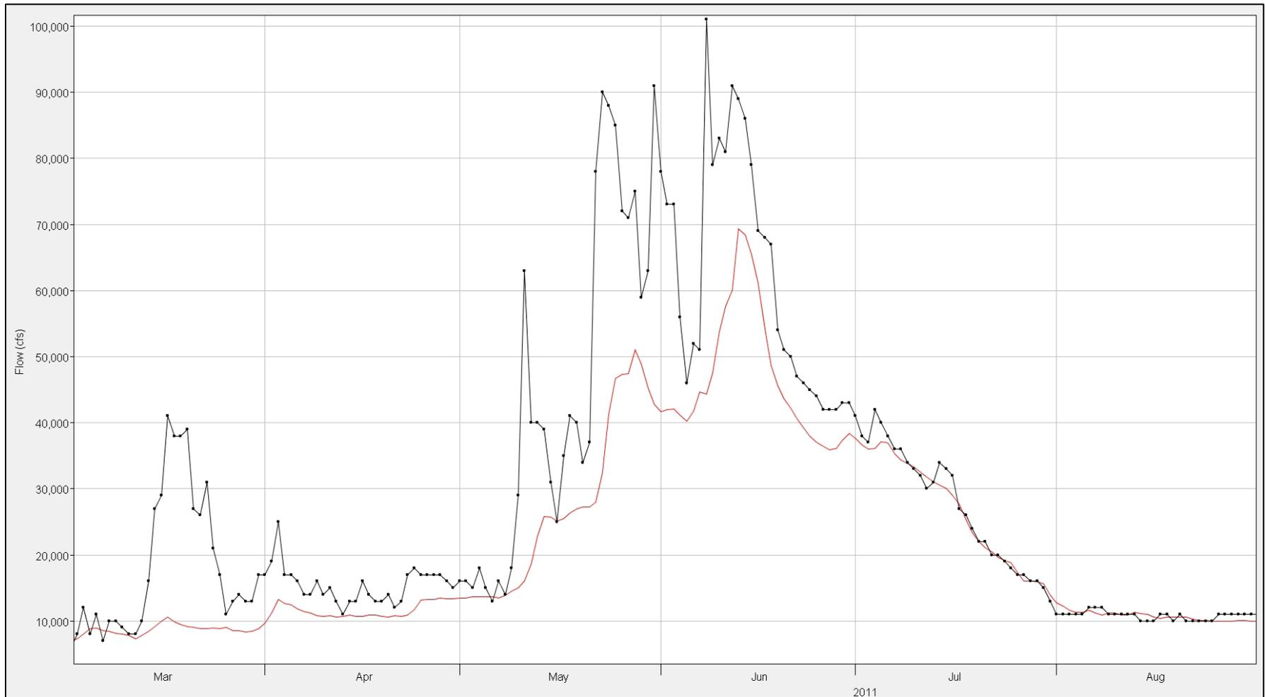
**Figure 8-13: Straddle-Stagger routing results for Landusky, MT-Fort Peck during 2011. Red data are the Straddle-Stagger data and black data are the observed data.**
