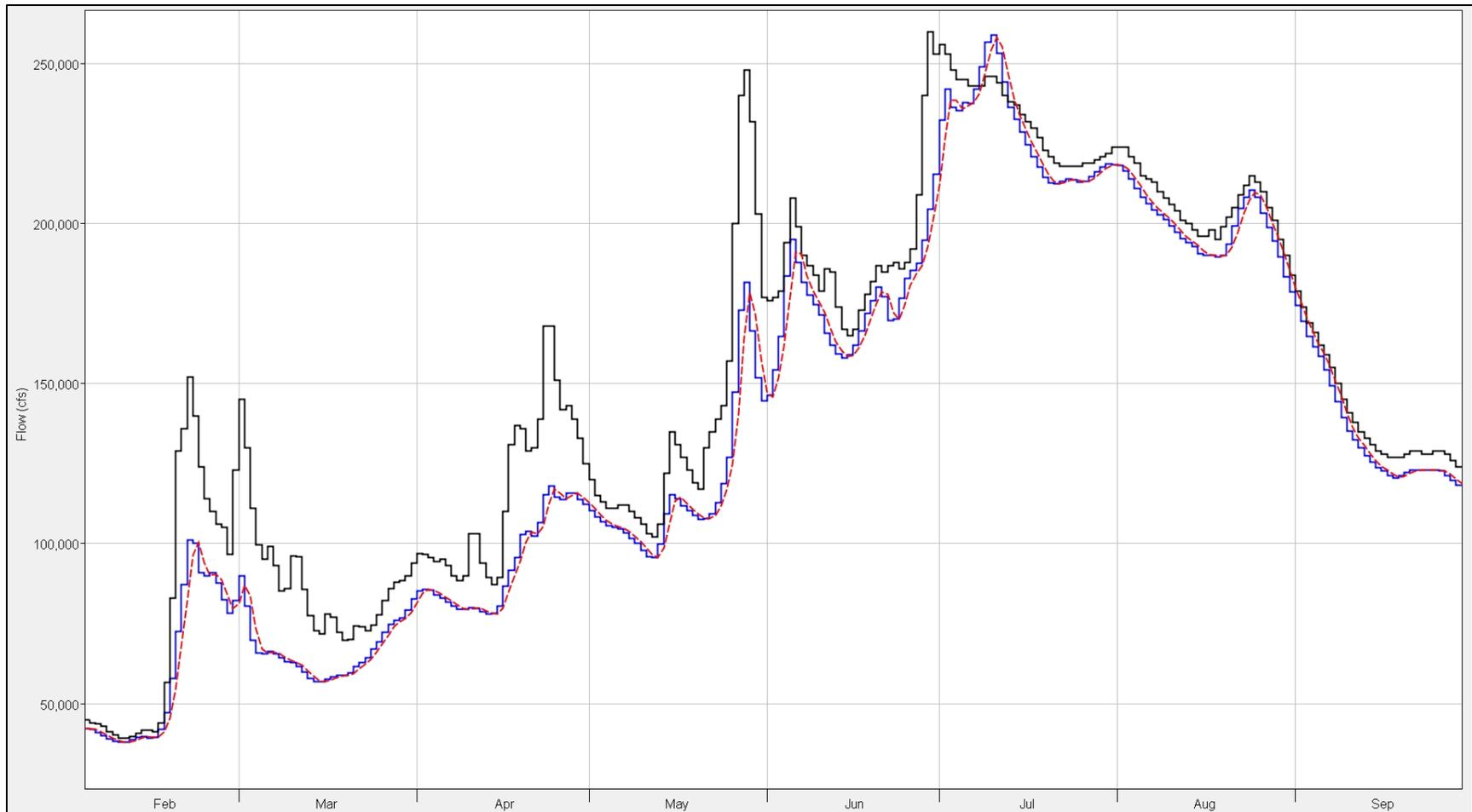
**Figure 8-47: Straddle-Stagger vs. Coefficient routing results for Waverly-Boonville during 2011. Red data are the Straddle-Stagger data, blue data are the Coefficient Routing data, and black data are the observed data.**
