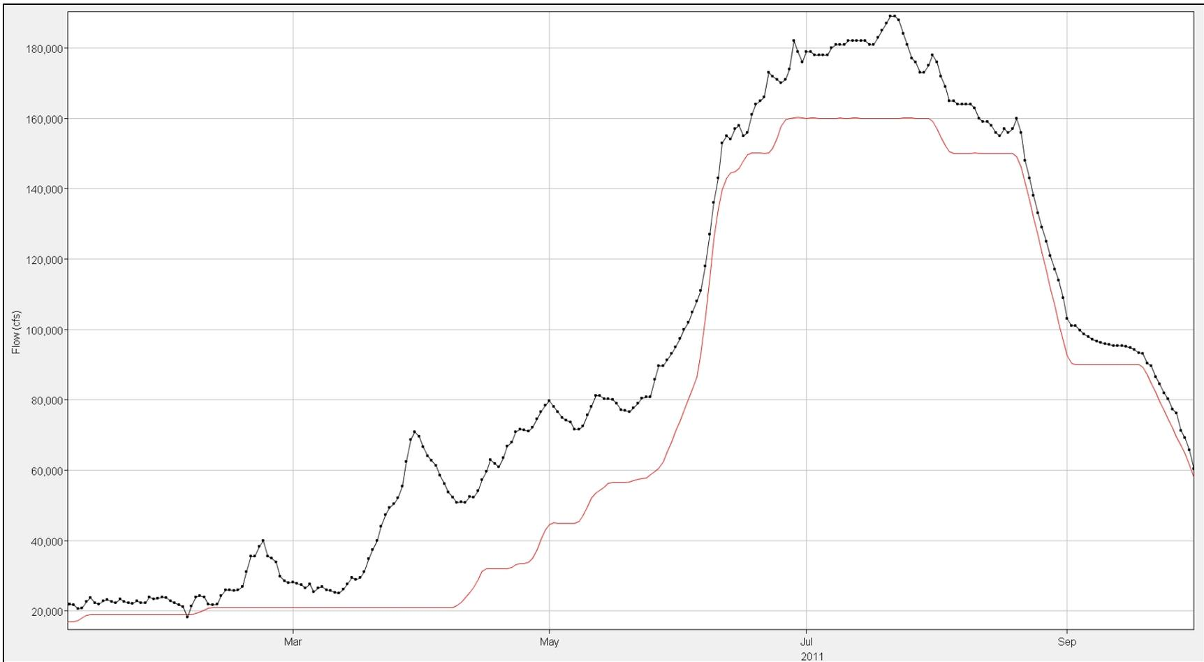
**Figure 8-22: Straddle-Stagger routing results for Gavins Point-Sioux City during 2011. Red data are the Straddle-Stagger data and black data are the observed data.**
