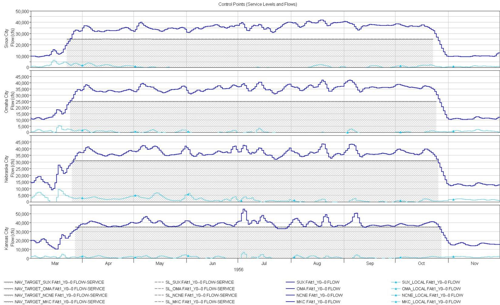
**Figure 5-26: Control points plot of target flows and simulated flows at each of the target locations.**
