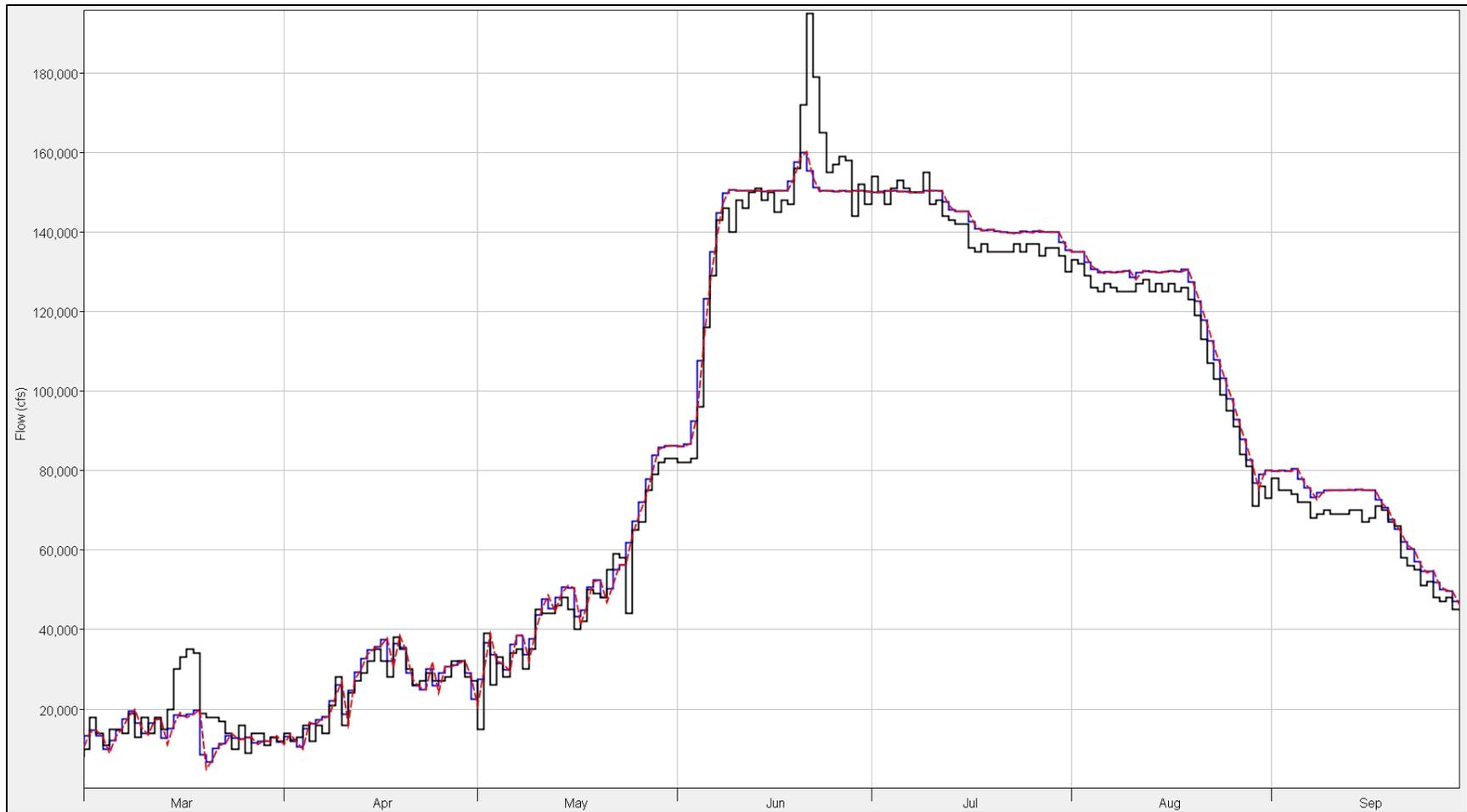
**Figure 8-37: Straddle-Stagger vs. Coefficient routing results for Oahe-Big Bend during 2011. Red data are the Straddle-Stagger data, blue data are the Coefficient Routing data, and black data are the observed data.**
