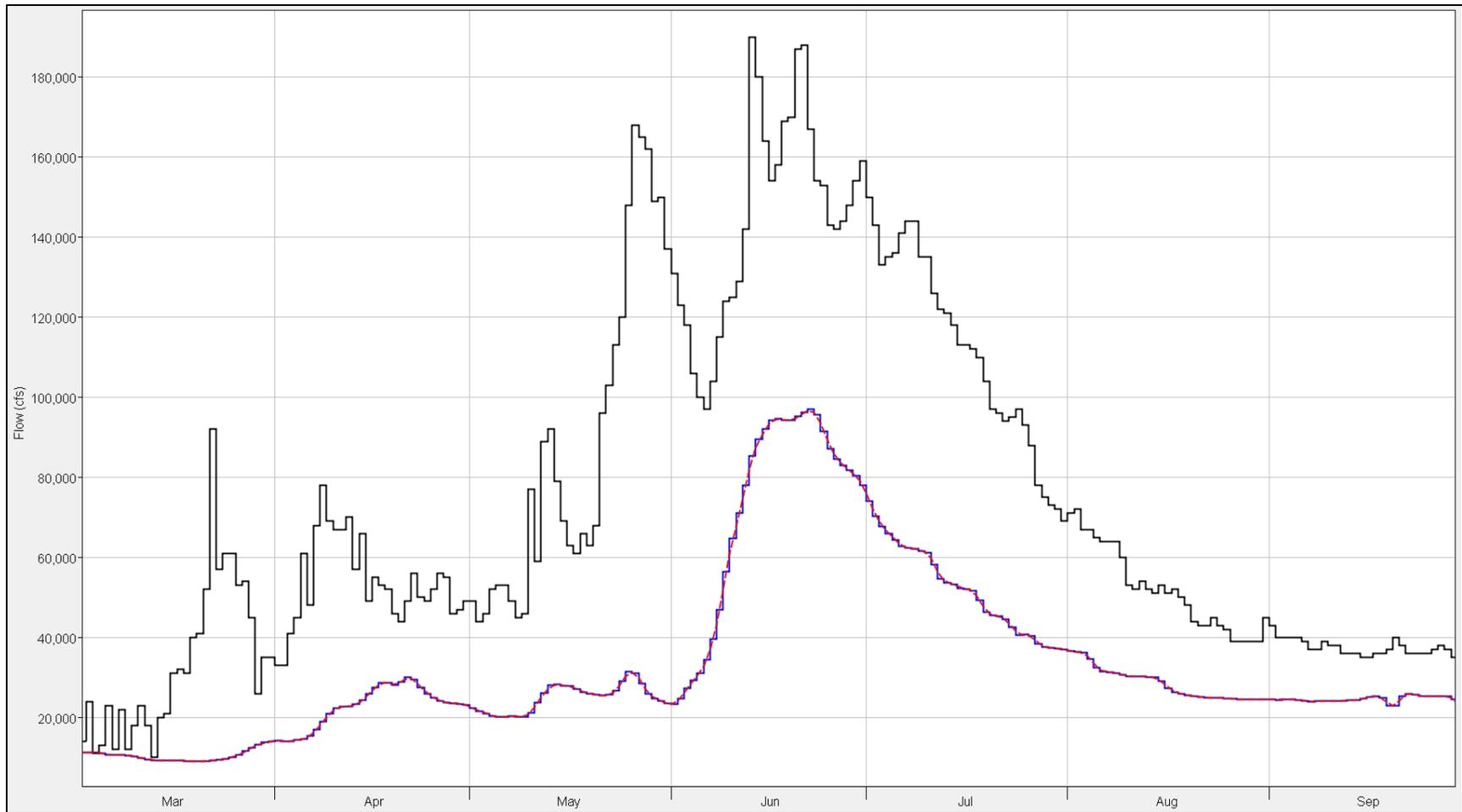
**Figure 8-34: Straddle-Stagger vs. Coefficient routing results for CLMT-Garrison during 2011. Red data are the Straddle-Stagger data, blue data are the Coefficient Routing data, and black data are the observed data.**
