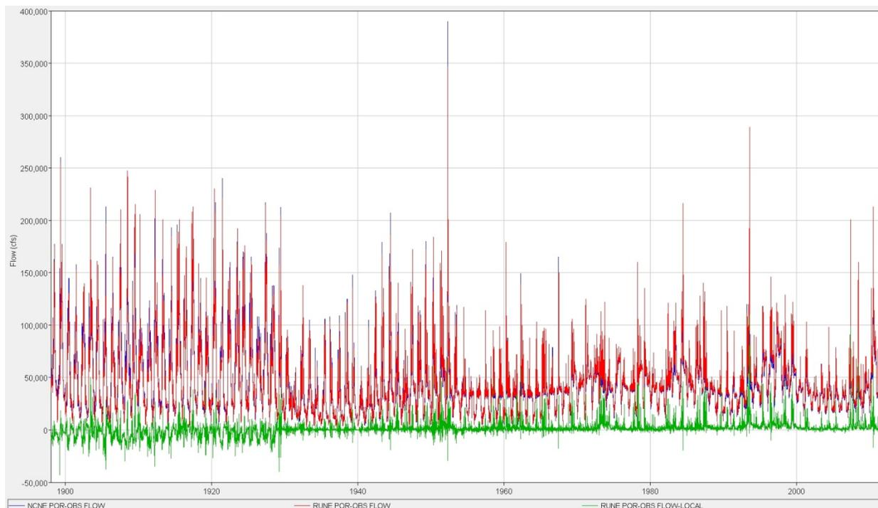
**Figure 3-3: Rulo unadjusted local flow for POR.**
