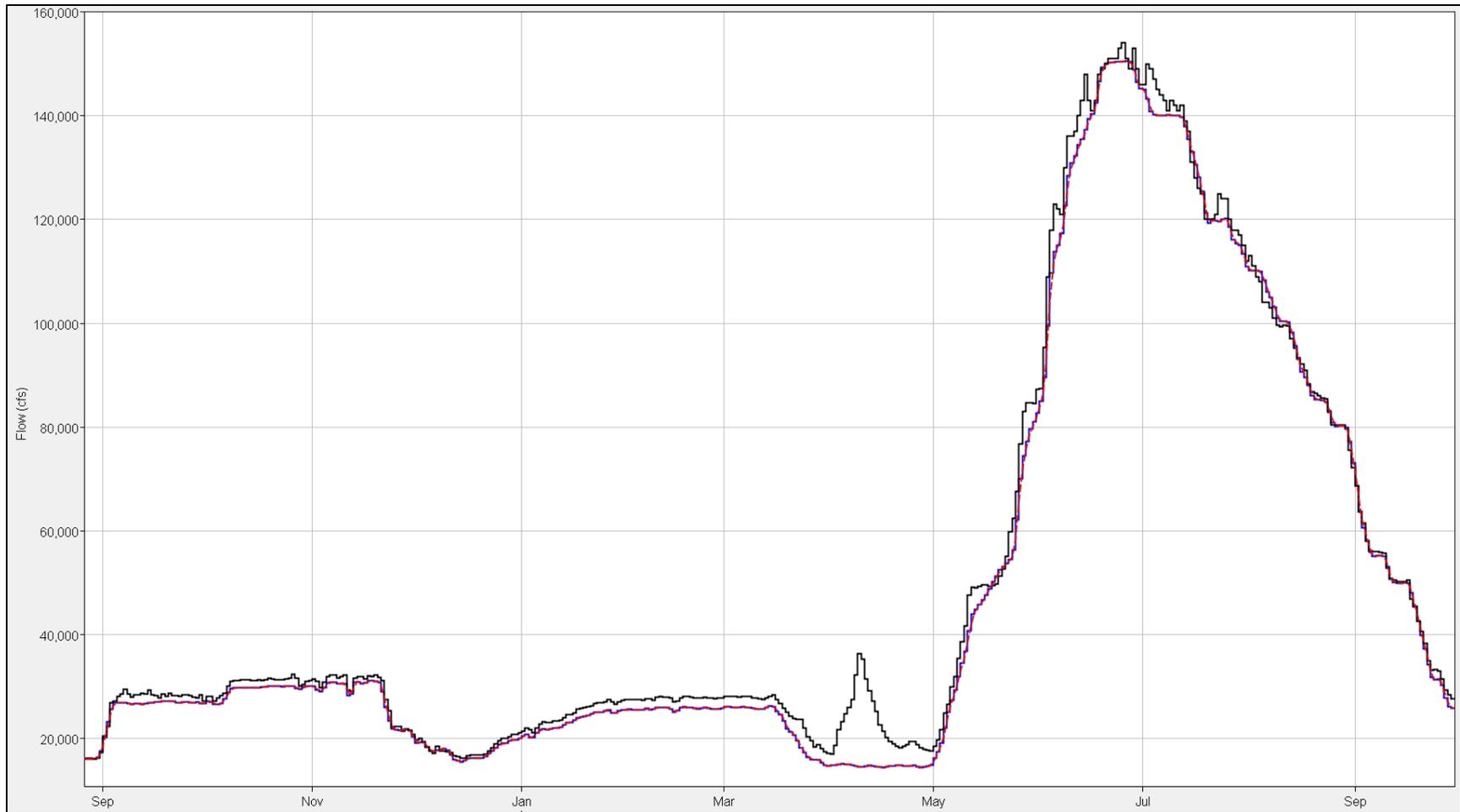
**Figure 8-35: Straddle-Stagger vs. Coefficient routing results for Garrison-BIS during 2011. Red data are the Straddle-Stagger data, blue data are the Coefficient Routing data, and black data are the observed data.**
