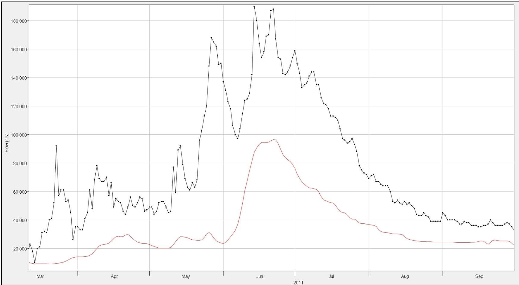
**Figure 8-16 Straddle-Stagger routing results for CLMT-Garrison during 2011. Red data are the Straddle-Stagger data and black data are the observed data.**
