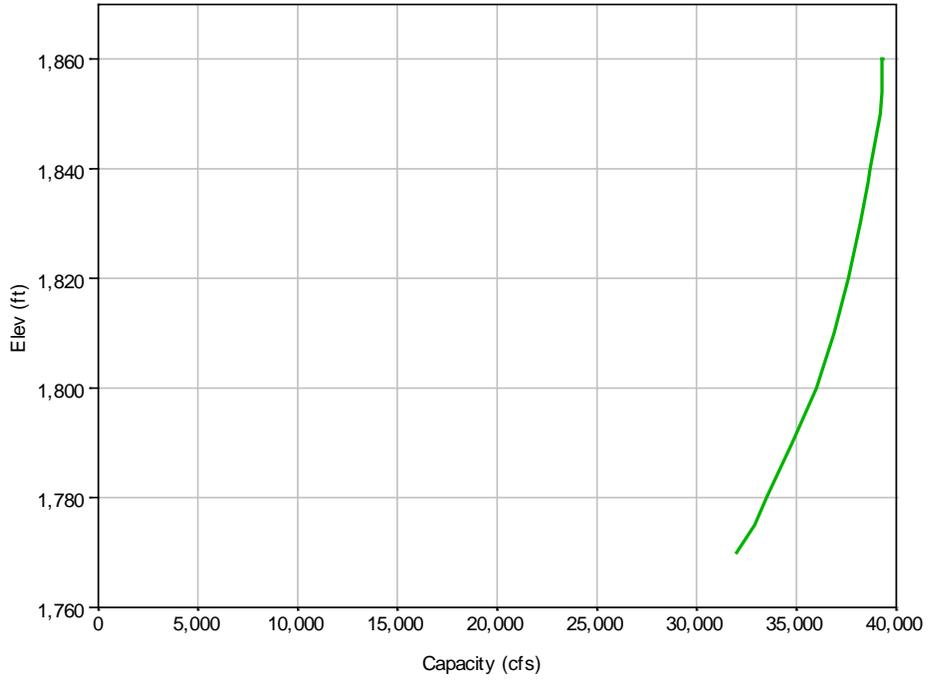
**Figure 3-17: Garrison powerhouse discharge capacity.**
