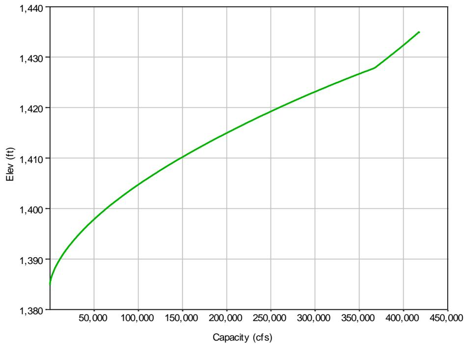
**Figure 3-10: Big Bend spillway capacity curve.**
