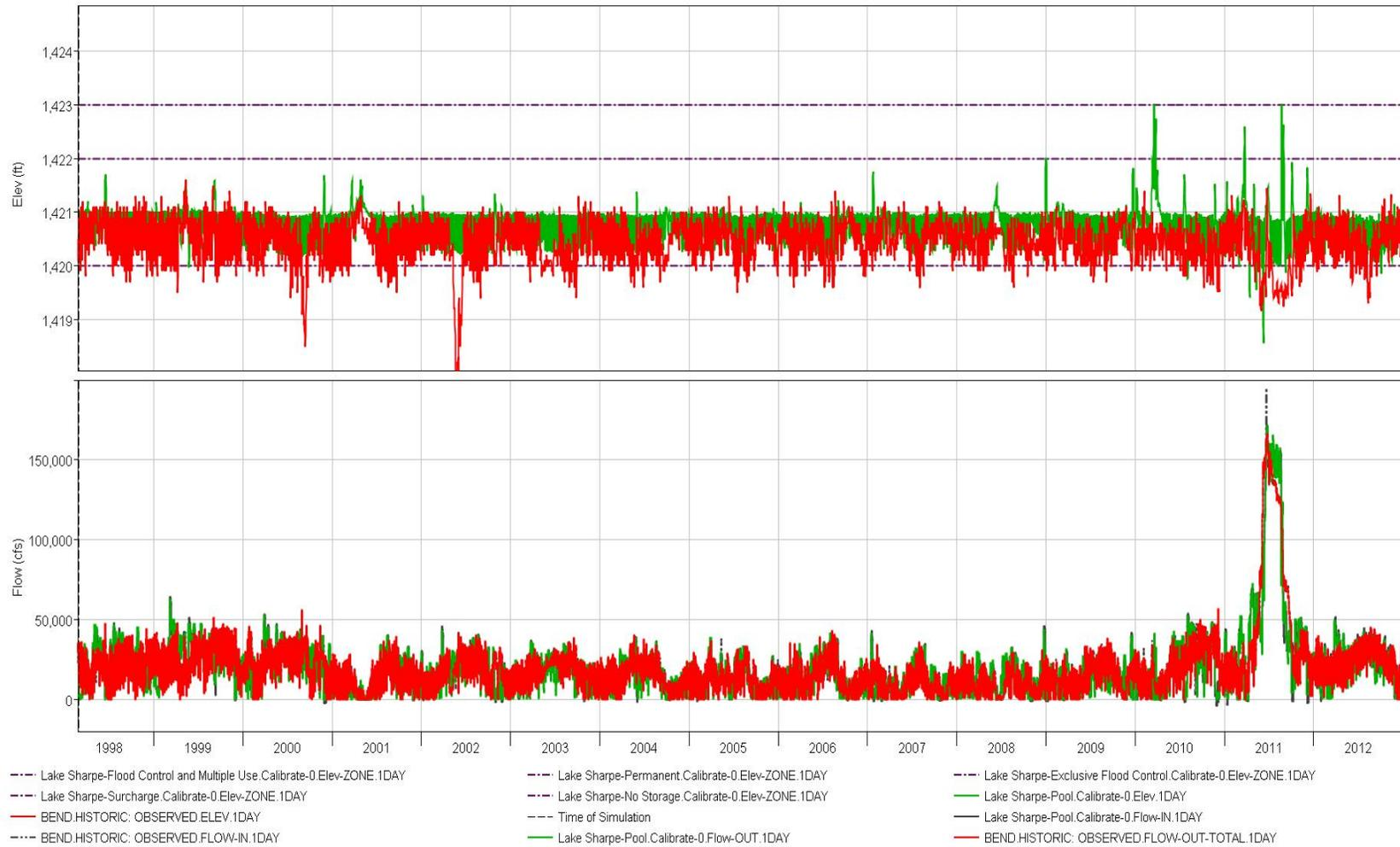
**Figure 5-4: ResSim versus historic operations at Big Bend Dam 1998-2012.**
