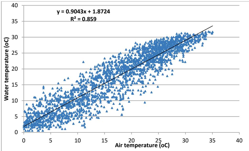
Seven year time series plot of observed and linear-regression-computed water temperatures with six day moving average air temperature at USGS 0689300 is presented in Figure 8.
