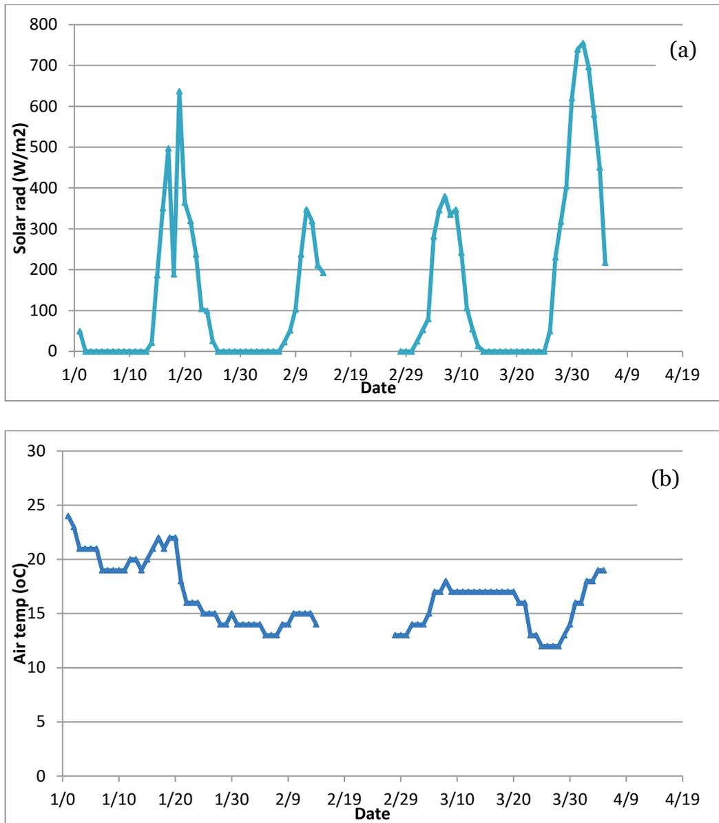
All gaps in meteorological data obtained from the above stations were linearly interpolated in HEC-DSS in order to use them as model inputs. Thus, the data gaps were filled with a straight line between the two bounding values. All meteorological data (after filling gaps) were compiled into one single HEC-DSS file (MoRmet.dss). For example, Figure 6 shows the time series plot of hourly air temperature at the Columbia Regional AP, MO station.
