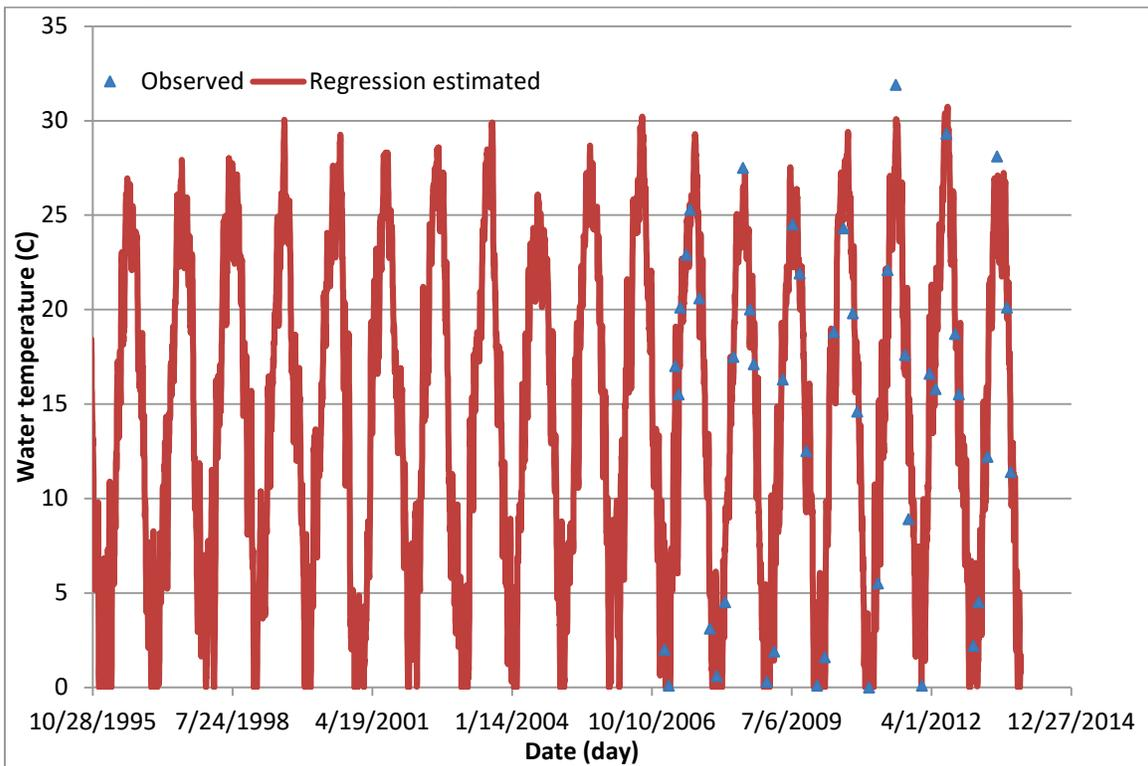
Figure C22. Regression computed versus observed water temperatures at BC22.
