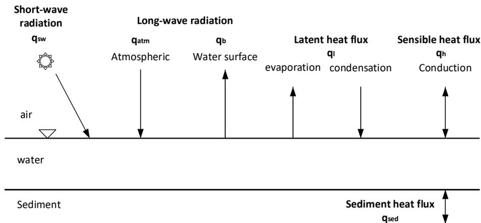
Units of heat flux ( $\text{W m}^{-2}$ ) are used to describe heat exchange at the air-water and sediment-water interfaces. The sign convention used herein is positive (+) for heat entering the water column, and negative (-) for heat leaving the water column. Net heat flux ( $q_{net}$ ) for the water column is
