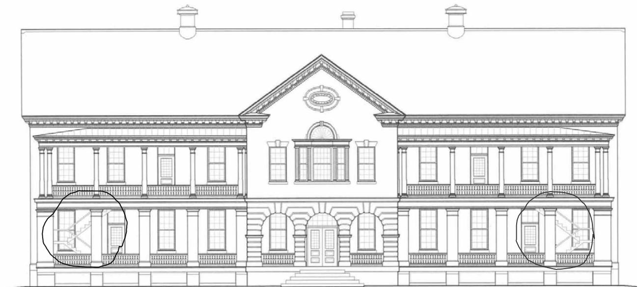
The new, fire egress stairs are visible only behind the main structure and detailing of the building. They are painted to blend in with the shadows of the porch.
