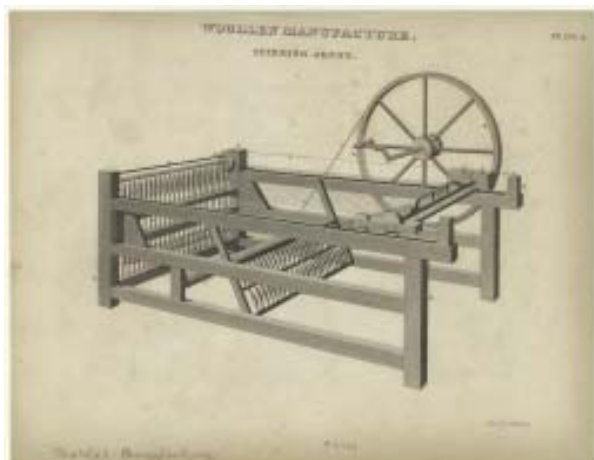
Woollen Manufacture : Spinning Jenny. The Picture Collection of the New York Public Library Source Note: From The cyclopedia: or, universal dictionary of arts, sciences and literature . (Philadelphia: Bradford, 1810-1842.) Rees, Abraham (1743-1825), author. Digital ID: 825894
