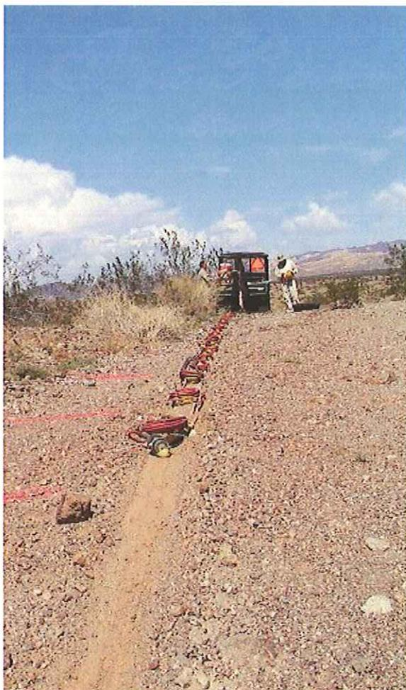
**Figure 2 - Towed Geophone Array**
