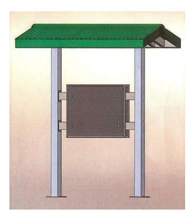
Frame legs to be installed such that the lowest portion of the panel is 28-32" from the ground surface. Approximately 30" of frame leg will be below the surface and encased in concrete to support the structure.
