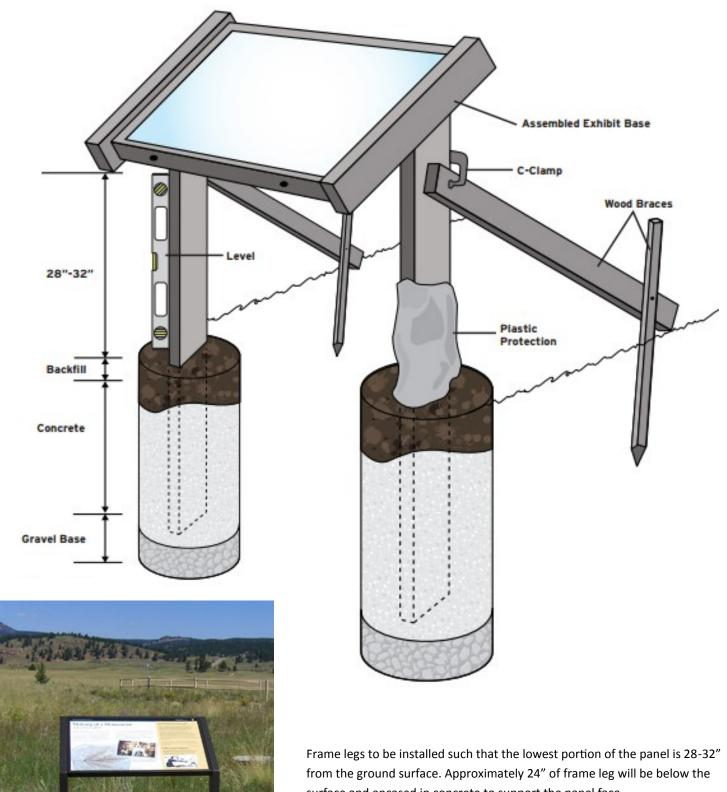
surface and encased in concrete to support the panel face.
