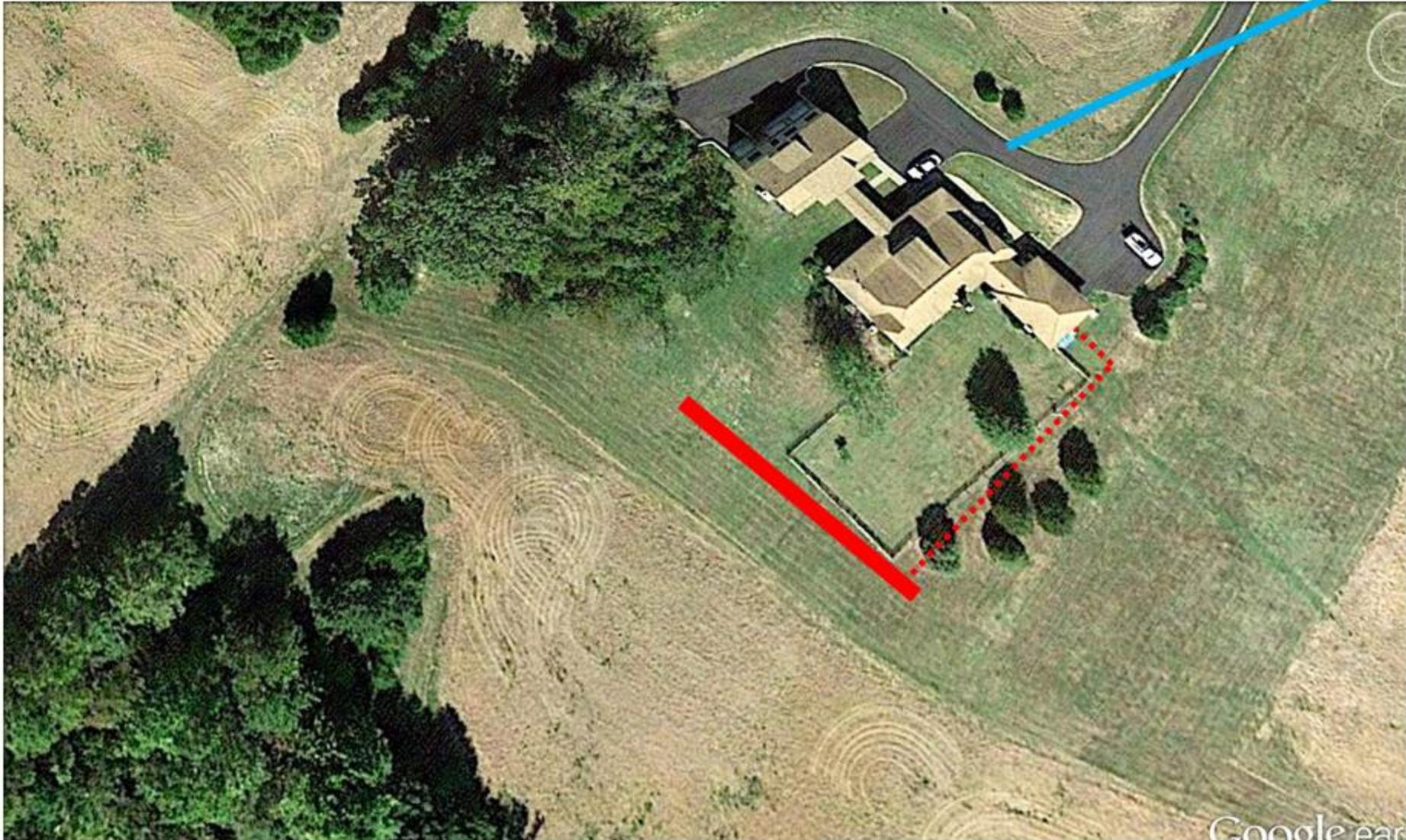
**solar-array (solid line): 117' length, 12' width, supported by 11 posts each 7' deep
