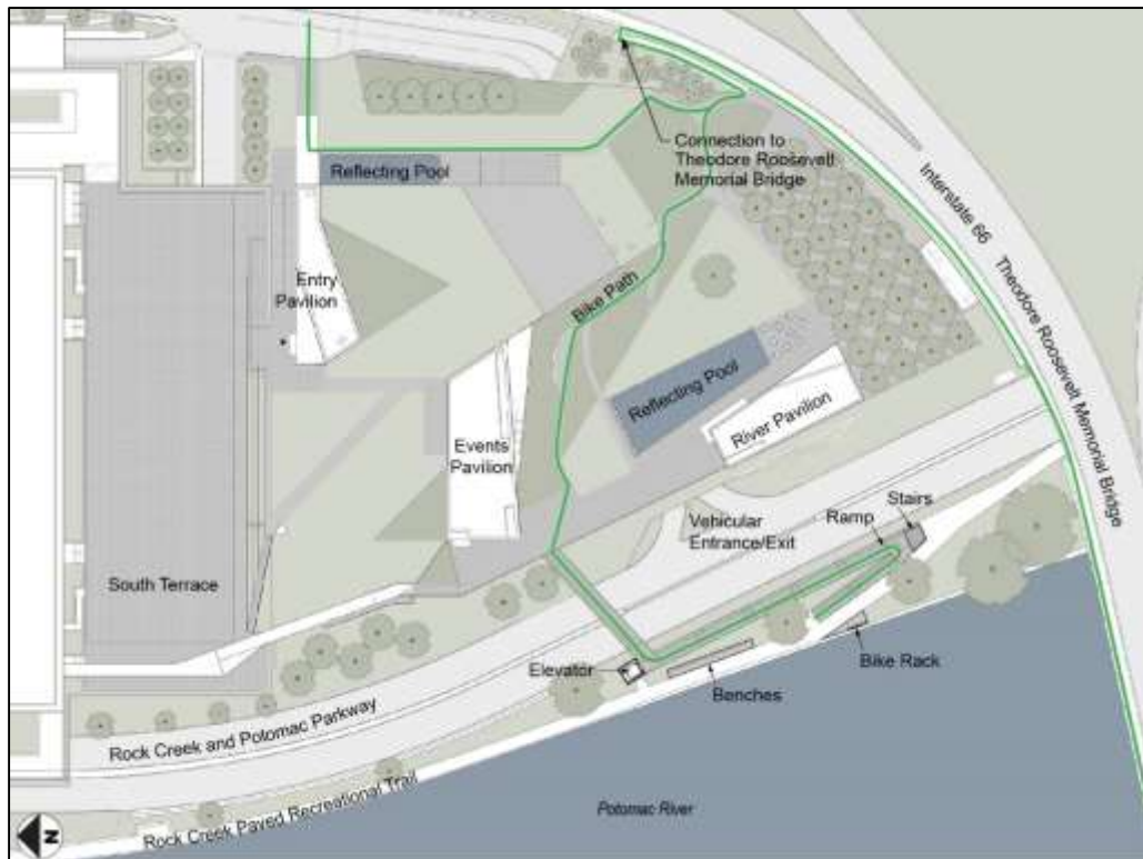
Figure 13: Bridge Access with Ramp and Elevator Alternative, plan view (not to scale) showing the proposed bicycle route (in green) from the Rock Creek Paved Recreation Trail through the site of the Expansion Project.
