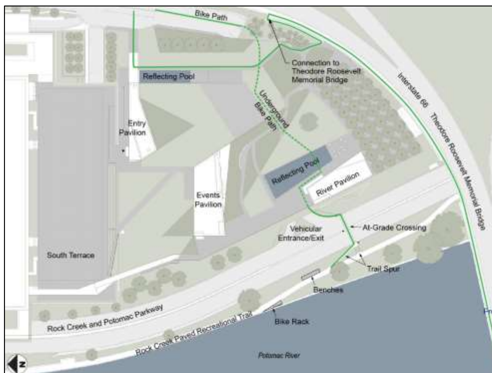
Figure 9: At-Grade Crossing Access Alternative, plan view (not to scale) showing the proposed bicycle route (in green) from the Rock Creek Paved Recreation Trail through the site of the Expansion Project.
