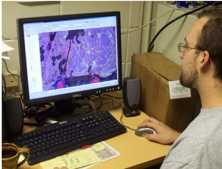
Figure 10. Trails were digitized from CIR DOQQs using heads-up digitizing techniques in ArcMap 9.1.
