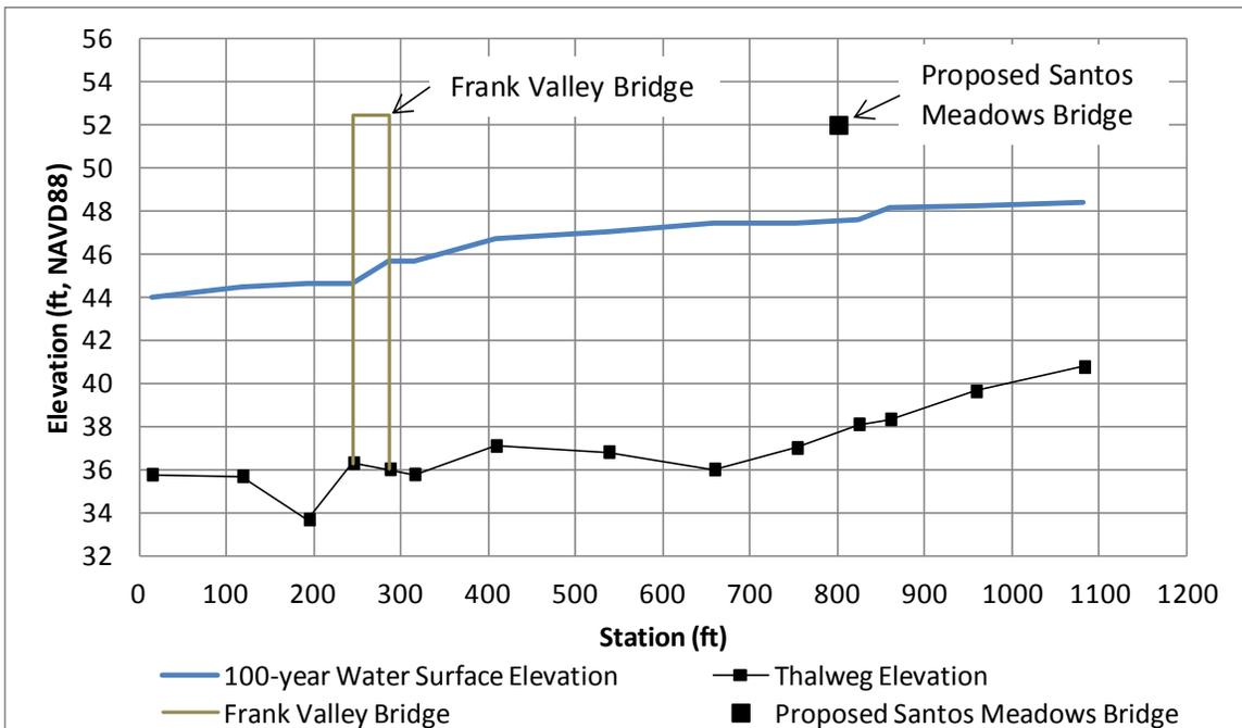
Figure 3. HEC-RAS model estimated 100-year peak flow water surface profile.
