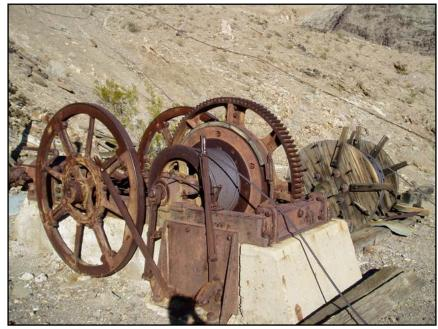
Photo 8. Hoisting engine and cable drum, a component of Structure 2 at Keane Wonder Mine (HRA 2006).
