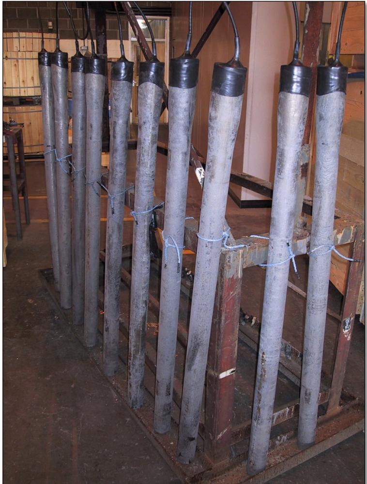
**Photograph 6.** High silicone cast iron anodes used with Alternative B.
