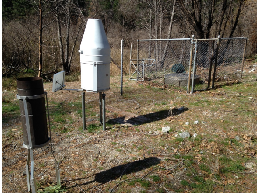
Figure 2: Manual precipitation gage (to be replaced, foreground), NOAA precipitation gage (will remain) and evaporation pan and fence (to be removed). The new precipitation gage and solar panel will occupy the same footprint as the old precipitation gage.
