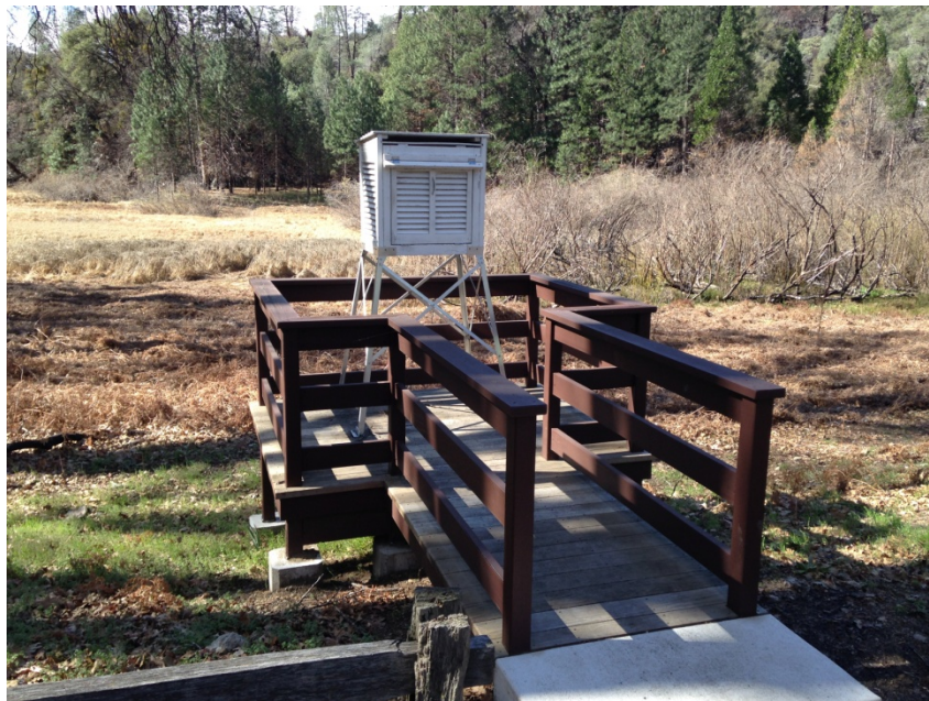
Figure 3: Temperature gage housing (will remain). A battery and radio will be added to box.
