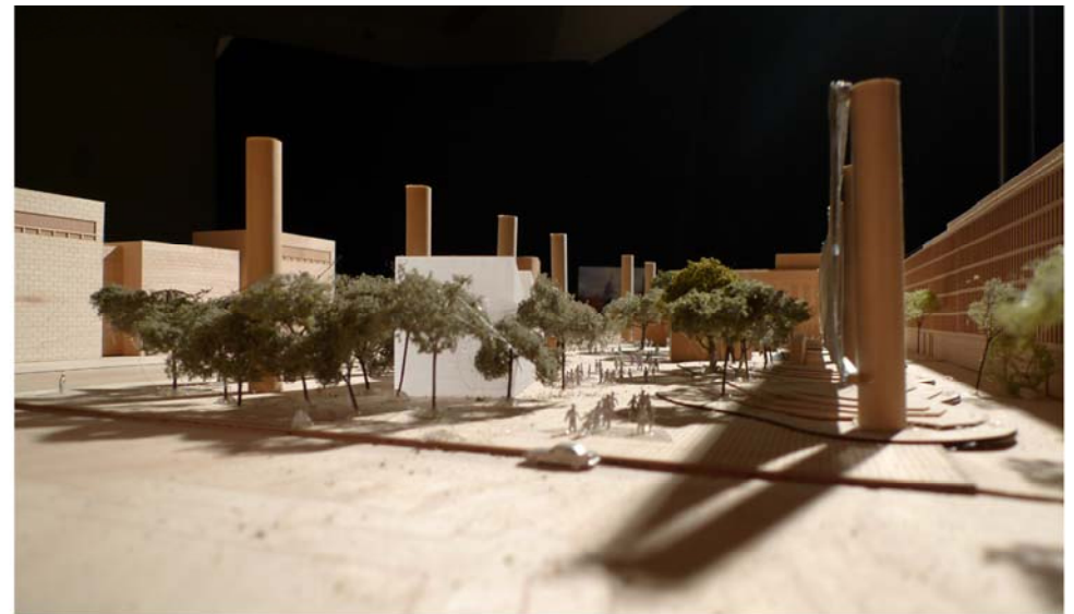
TAPESTRY/COLUMN STUDY WITH 10' DIAMETER COLUMNS AND SOUTH TAPESTRY ONLY AT 80' HEIGHT.
