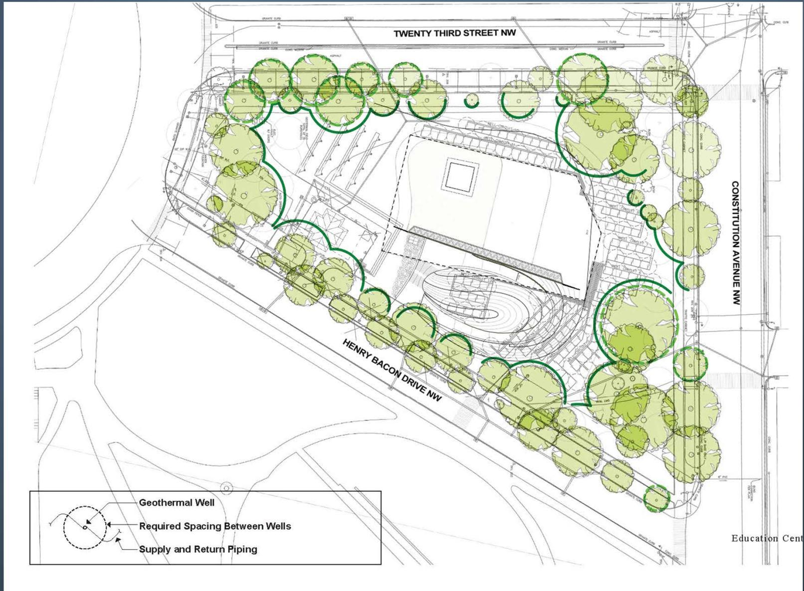
Visitor Center has been designed to minimize any damage to existing trees on the site and also incorporates geothermal wells in order to reduce the need for visible mechanical equipment
