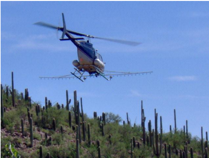
Figure 13. Helicopter with boom sprayer.
