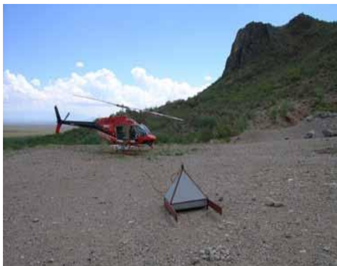
“Pyramid housing” nozzle assembly (US Forest Service)
