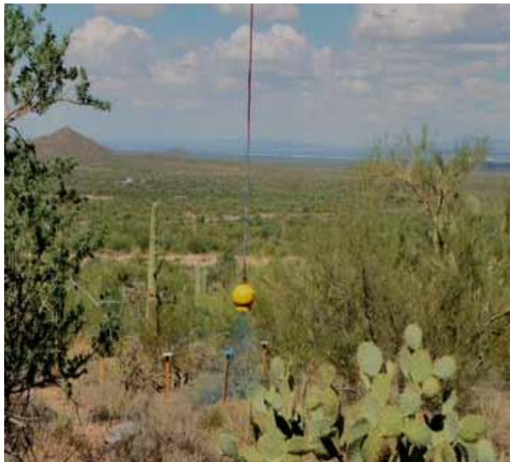
Test spraying with “spray ball” nozzle assembly (US Forest Service)
