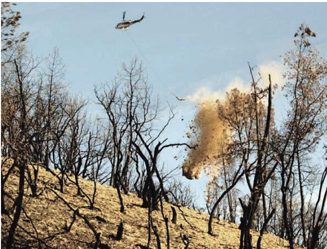
Figure 14. Helicopter delivering mulch to mitigate soil erosion after an intense fire in the western United States.
