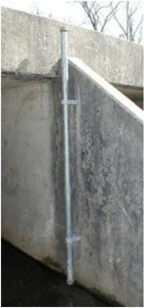
Example of crest stage gage to be installed at each culvert with crossing structure. Photo courtesy of Paul Rydlund.
