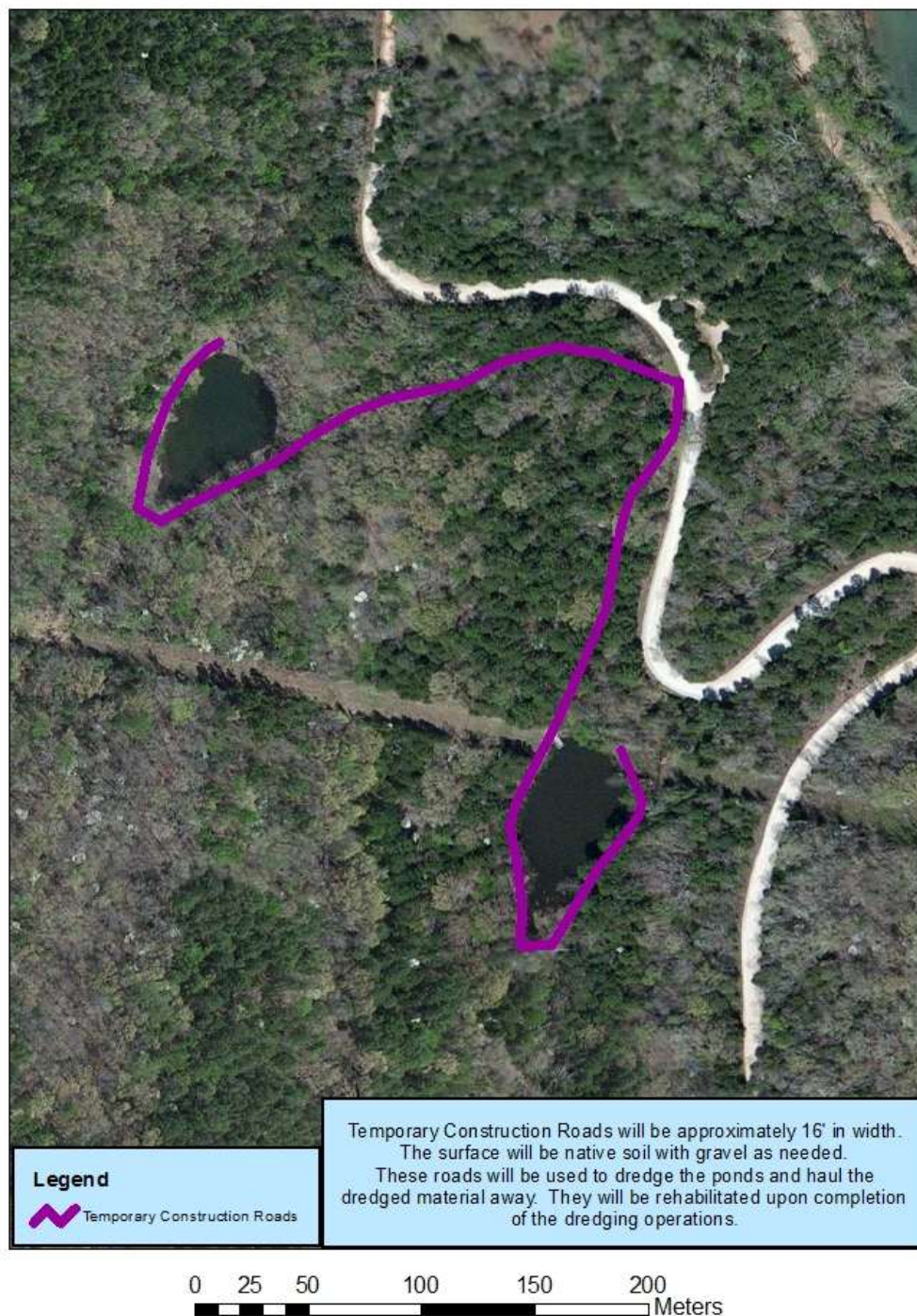
Figure 5. Temporary construction roads for dredging the ponds.
