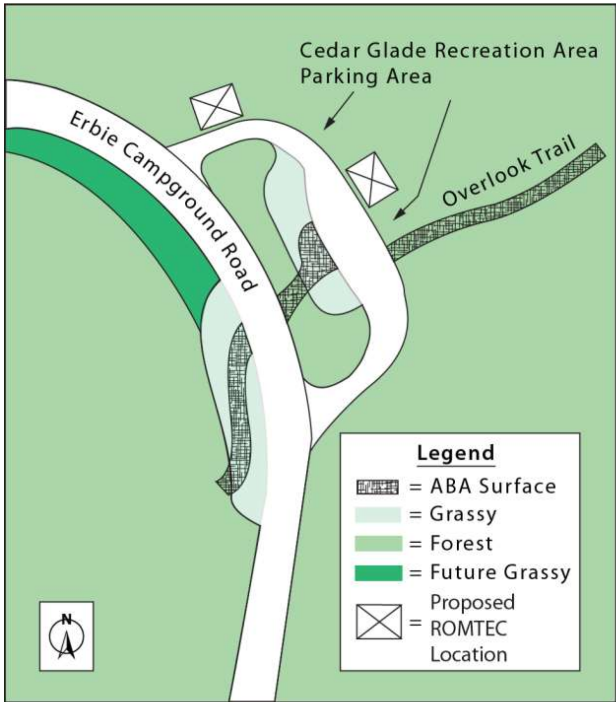
Figure 2. Proposed locations of ROMTEC bathroom and hardened surfaces for barrier-free compliance.
