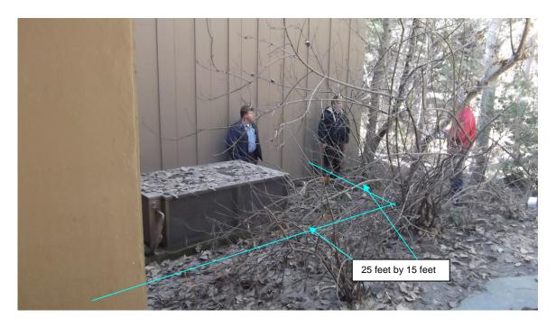
Proposed breezeway area for new cooling tower placement. Note that ground disturbance will only occur within this notch in the Village Store building which is approximately 25 by 15 feet.
