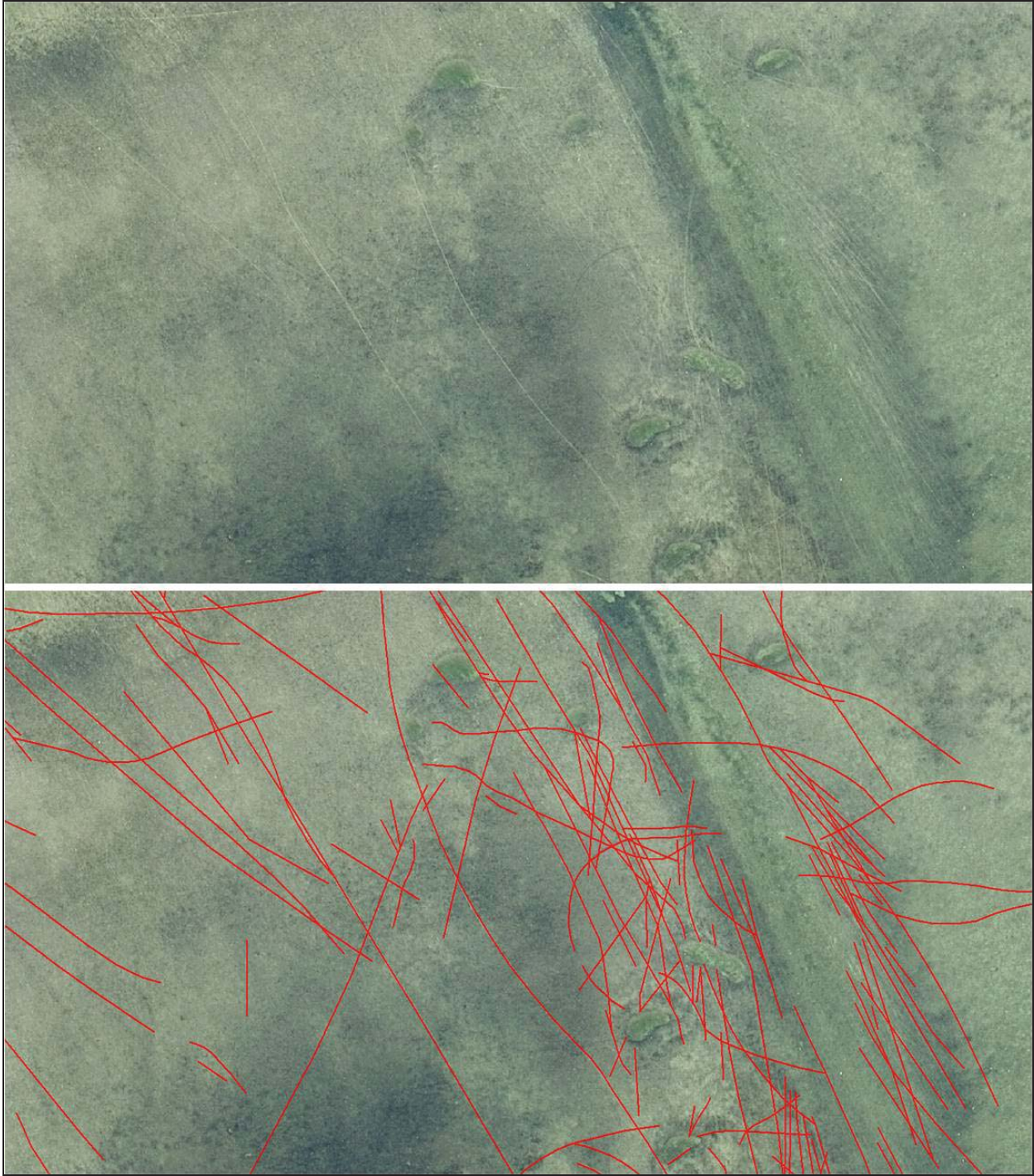
Figure 7. An illustration of the prop scar digitization process using images from Treatment Area 2. The potential prop scars visible in the top image have been mapped in red in the bottom image. Image scale is 1:1000.
